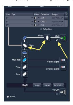
Select an appropriate emission filter for the AiryScan channel. Note, most of these are dual pass filters. Select the one most suitable not only for detection of your fluorophore, but also for rejection of unwanted emissions.
