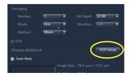
Set the capture Bit Depth and Scan Direction. The default for the AiryScan is an 8 bit, bidirectional scan. Twelve bit and single direction capture can be used, if desired.
