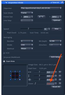
At this time note the AiryScan Multitrack ILEX Setup button. This is for purely SR multitrack imaging and requires a slightly different workflow. This will be covered in a separate section, below.
