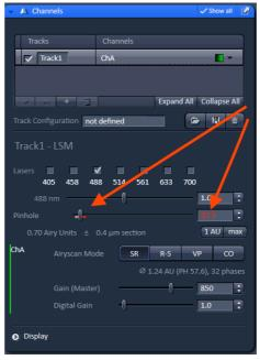
Set and optimize the exposure. You must use the range indicator to ensure there are no saturated (overexposed) pixels. Note the AiryScan does not present an adjustment for offset (black level).
