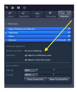
Return to the "Acquisition" window and click on "Continuous Scan". Alignment may take 30 seconds or more. The "AiryScan" panel you have undocked will show "Quality and Status" messages such as "No Beam (Waiting)" "Analyzing" and "Good (Waiting)". The latter, displayed in green, indicates correct alignment. The Detector View display should update to show a more balanced illumination. Close the "AiryScan" panel (this will return to the "Maintain" window).
