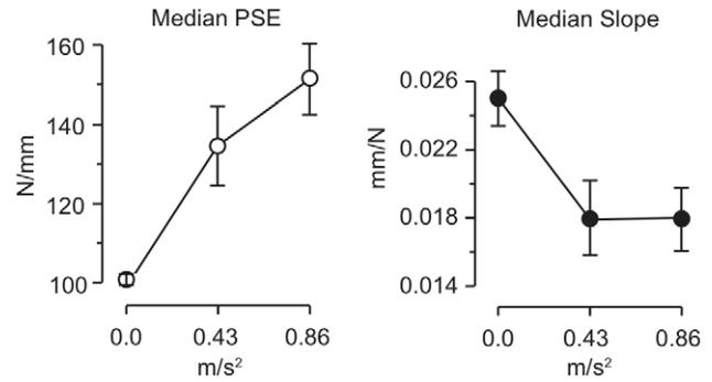
**Figure 8.** Experiment 2: Median values of the PSE and slope from per-subject psychometric fits at each vibration amplitude level. Error bars: ± 1 SEM (outliers excluded). doi:10.1371/journal.pone.0017697.g008
