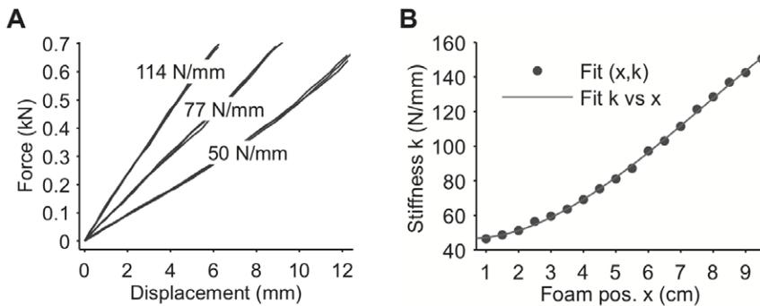
**Figure 4. Force-displacement profiles and fits of stiffness vs. foam position used to calibrate the apparatus.** A. Examples of three compression profiles are shown (overlaid) for each of three stiffness values. Each calibration was based on sixty such profiles, with more than 3000 data points each. B. Calibration curve fit of stiffness vs. foam position based on measurements at each position and stiffness. doi:10.1371/journal.pone.0017697.g004
