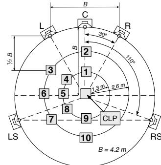
FIGURE 5 – Listening positions in Experiment A.
