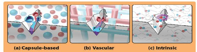
Figure 1. Self-healing polymers have been demonstrated using three conceptual approaches including (a) capsule-based, (b) vascular, and (c) intrinsic mechanisms.
