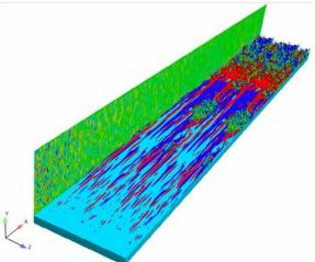
Figure 1: Snapshot of a boundary layer undergoing bypass transition beneath free-stream turbulence. Red and blue isosurfaces are high- and low-speed streaks. Localized turbulent spots are identified by isosurfaces of the  $\lambda_2$  criterion.
