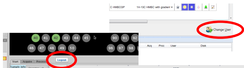
Figure 1. Change User (Bruker) and Logout (Varian) buttons. If you cannot see the Logout button on the Varian, go to the Start panel.
