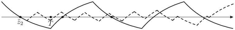
Fig. 11 A graph of one solution for case FNFP , where the parameters are \tau = 1, \sigma = 0.35, \beta_U = 0.3, \beta_L = 0.4, a = 0.7 , and \Delta = 2.22 , suggesting that for certain values of the parameters the solution x^{(\Delta)} might settle down on a rapidly oscillating periodic solution, in which case we would have T(\Delta) = \infty
