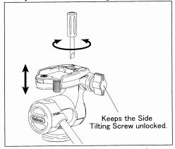
Rotate the screw as seen in the drawing, Camera plate moves slightly up or down.
