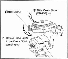
Rotate Shoe Lever until the Quick Shoe raises up automatically. Slide it out from the head then attach to the bottom of camera body. Then screw in carefully and tighten with a camera firmly.
