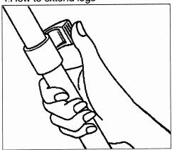
Using thumb to open the Leg Locking Lever to extend leas to the desired height. Then locking each leg section firmly. For the folding legs, opening the Leg Locking Lever and collapse from the lower leg section to the upper leg section.
