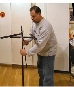
Next, place the boom arm onto the stand's vertical pipe, and twist the stand's pipe until its threads are seated firmly into the boom arm. Note that the center U-channel opens toward the bottom, and the two side U-channels are open on the top.
