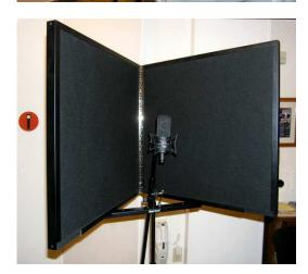
Finally, adjust the boom arm so the microphone is about halfway up and centered inside the Portable Vocal Booth. When you're all done it should look like the photo at left.
