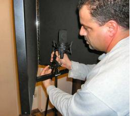
Next, attach the microphone's shock mount (or standard mount) onto the end of the boom arm just as you would without the Portable Vocal Booth. We suggest that you loosen the boom arm's locking knob and twist the boom arm to screw it into the microphone base. This is much easier than rotating the microphone!
