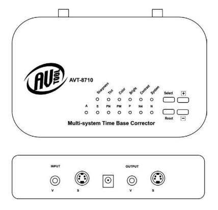
Connect the AC to +12 VDC adapter to an AC source and then to the DC power input shown in the middle of the lower drawing above. (Note that there is no power switch. The unit will begin to work as soon as you have the AC to +12 VDC adapter plugged in and furnishing power).
