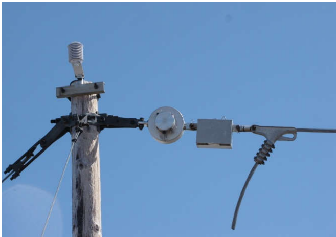
Fig. 5 The next generation: The conductor is connected at the top to a mechanical dynamometer (rectangular box) and a load cell with a digital recorder (circular box). A digital thermometer is on top of the pole, at the same height as the measuring wire.
