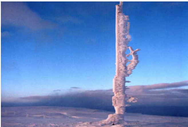
Fig. 6 At some of the test spans Landsnet also operates weather stations, this one is in East-Iceland. Here it is covered in icing, and the anemometer is frozen.
