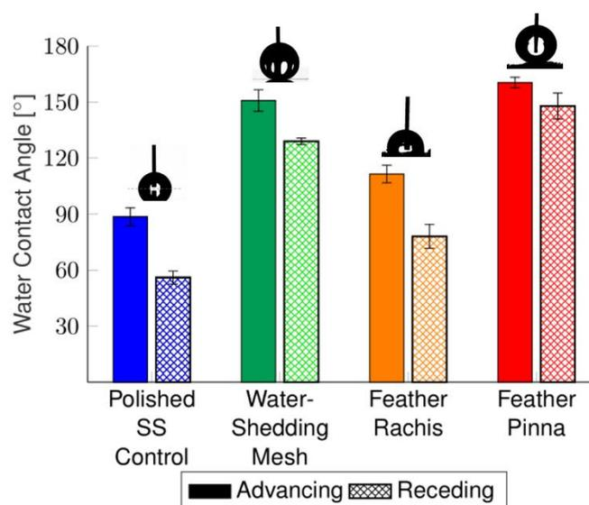
Fig. 3 Advancing and receding contact angles measured on the: polished stainless-steel control, smooth feather rachis, hierarchically textured feather pinna, and water-shedding biomimetic mesh surfaces. No wettability data are presented here for the water-wicking mesh surface as water droplets present with contact angles of 0°, completely wetting the surface. Error bars show 95% confidence intervals on the mean.
