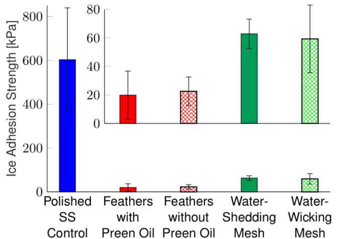
Fig. 4 Ice adhesion strength measured on the: reconstructed plumage mat with preen oil, reconstructed plumage mat with preen oil removed, water-shedding biomimetic stainless-steel mesh, and water-wicking stainless-steel mesh in comparison with a flat polished stainless-steel control sample. Error bars shown 95% confidence intervals on the mean.
