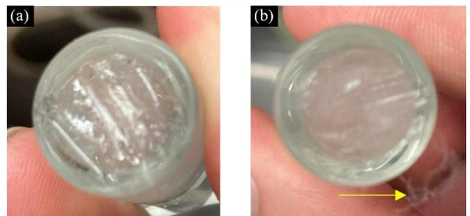
Fig. 5 (a) Underside of an ice column dislodged from the reconstructed plumage mat showing the imprint of the once adhered penguin feathers. (b) A dislodged ice column with a small feather piece attached to it.
