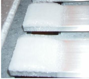
Fig. 5 Typical Ice Deposit in Cold Room at -8°C
