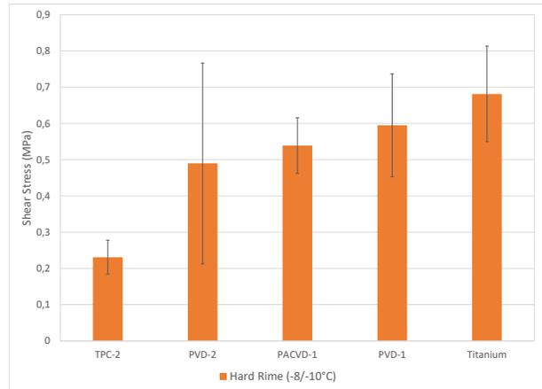
Fig. 11 Shear Stress Comparison obtained under hard rime in Cold Room for coating applied on titanium substrates
