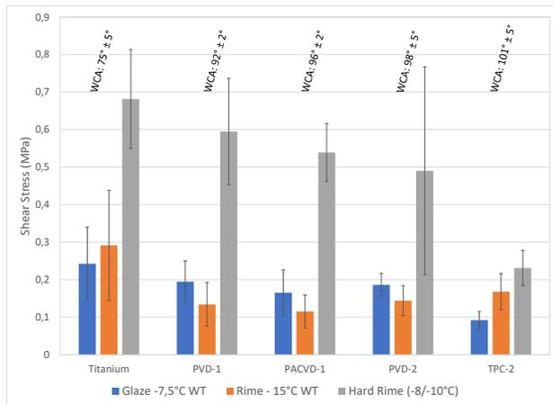
Fig. 13 Shear Stress Comparison Coatings applied on Titanium substrate classified according to their contact angle
