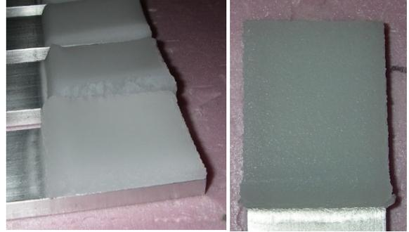
Fig. 3 Typical Ice Deposit in Wind Tunnel at  $-15^\circ\text{C}$  with Wind Speed set to 50 m/s
