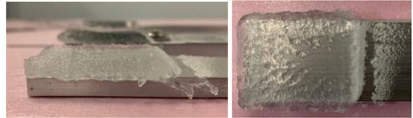
Fig. 4 Typical Ice Deposit in Wind Tunnel at  $-7.5^\circ\text{C}$  with Wind Speed set to 55 m/s
