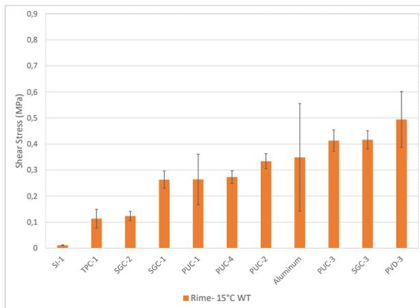
Fig. 6 Shear Stress Comparison obtained under rime in wind tunnel for coating applied on aluminum substrates
