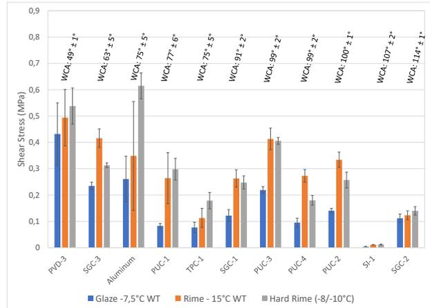
Fig. 12 Shear Stress Comparison Coatings applied on Aluminum substrate classified according to their contact angle
