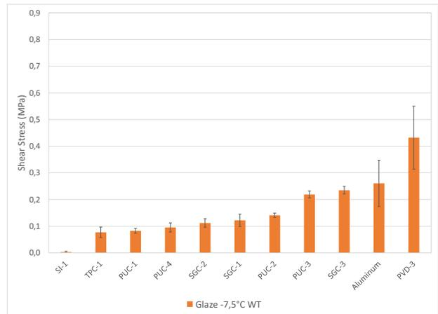
Fig. 8 Shear Stress Comparison obtained under glaze in wind tunnel for coating applied on aluminum substrates
