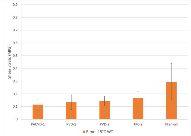
Fig. 7 Shear Stress Comparison obtained under rime in wind tunnel for coating applied on titanium substrates
