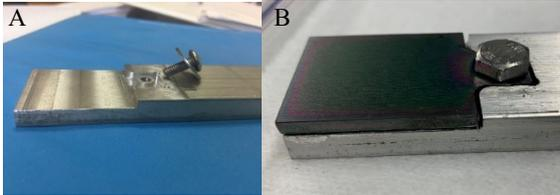
Fig. 2 CAT Sample (A) and Embedded Test Coupon (T6AV) (B).
