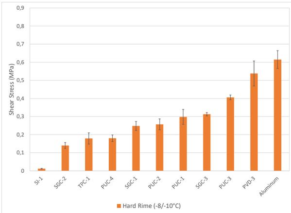
Fig. 10 Shear Stress Comparison obtained under hard rime in Cold Room for coating applied on aluminum substrates
