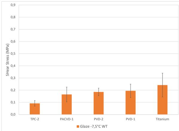
Fig. 9 Shear Stress Comparison obtained under glaze in wind tunnel for coating applied on titanium substrates
