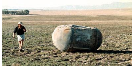
Recovered Delta second stage propellant tank
