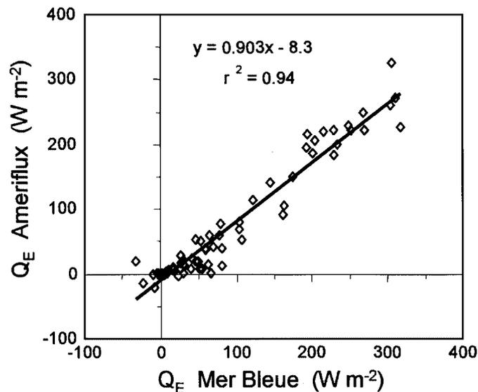
Figure 1. Comparison of 30 min latent heat flux  $Q_E$  measurements from the Mer Bleu eddy-covariance measurement system using an open-path hygrometer against the AMERIFLUX roving closed-path eddy-covariance system. Data are from June 2001
