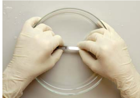
under water: run the rod across the cutting edge
