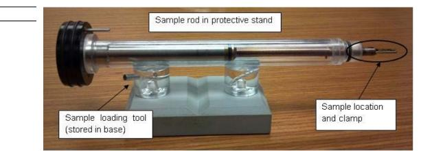
a. Using one hand to prevent the holder from slipping out of the stand, INSERT the loading tool into the hole in the specimen clamp and GENTLY RAISE the clamp straight up until it stops. NEVER use tweezers.
