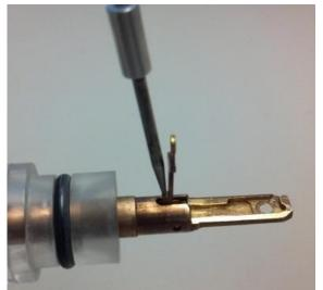
e. Use the microscope to inspect the holder Oring for debris. Gently remove any debris using a sheet of Kimwipe.
