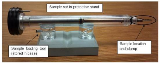
iii. Using one hand to prevent the holder from slipping out of the stand, INSERT the tool into the hole in the specimen clamp and GENTLY RAISE the clamp straight up until it stops.
