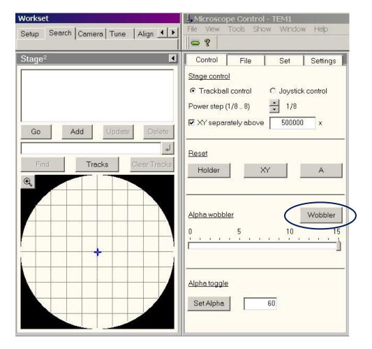
c. Once the Eucentric Height is completed, DEVACTIVATE the Alpha Wobbler by PRESSING the L3 button or the Wobbler button on the Stage flap-out window.
