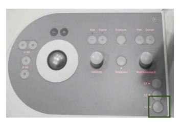
the Left-Hand Control Pad. Alternatively, you may PRESS the Wobbler button on the Stage control window. The stage will automatically rock through a tilt range of +/- 15°.
