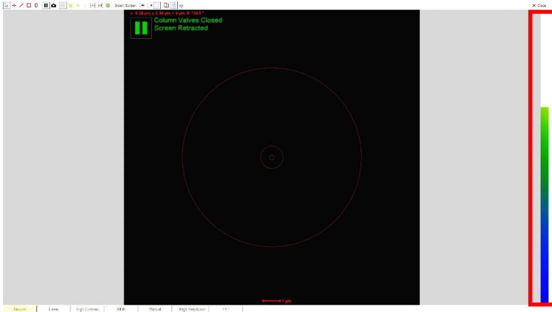
Figure 32 FluCam interface. The beam intensity is shown at the right of the window. Red means a higher intensity, and blue for a lower intensity.
