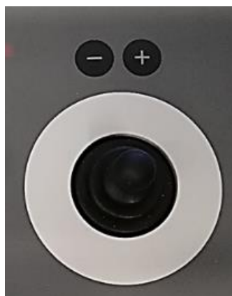
Figure 24 Image of the joystick for moving the sample. Use (-) or (+) to decrease or increase the movement, respectively.
