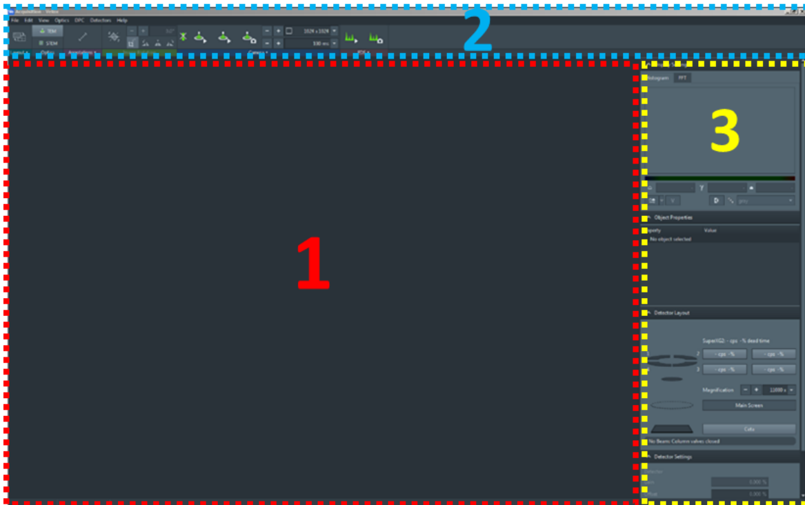
Figure 5 Layout of the Velox software in acquisition mode, showing the three main parts: the imaging viewer (red), the imaging options (blue), and the settings (yellow).
