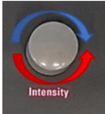
Figure 4 Increasing (red) or decreasing (blue) the beam intensity on the Microscope.
