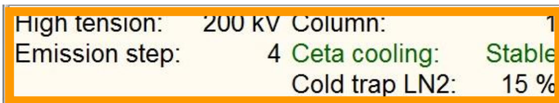
Figure 11 Status displays where the high tension and ceta cooling values and status can be found.
