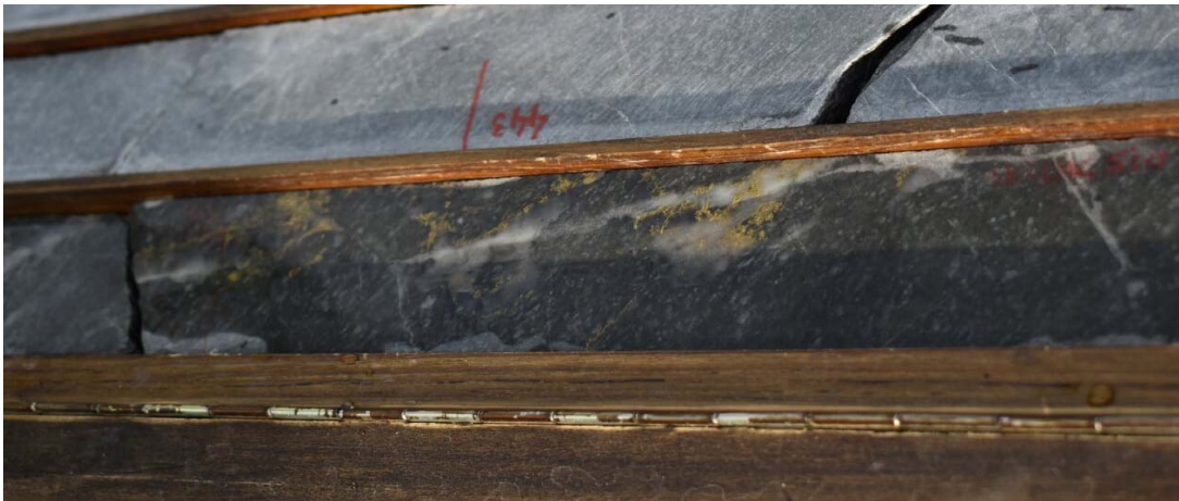
Figure 4. Visible gold in diamond drill core at North Mara Gold Mine
