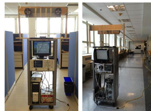
Figure 6: Carrying out channel measurement for static environment in corridor
