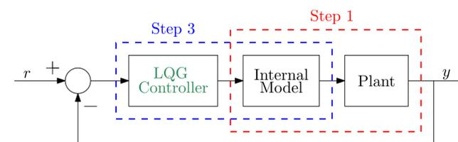
Figure: Controller Synthesis Method, Steps 1-3
