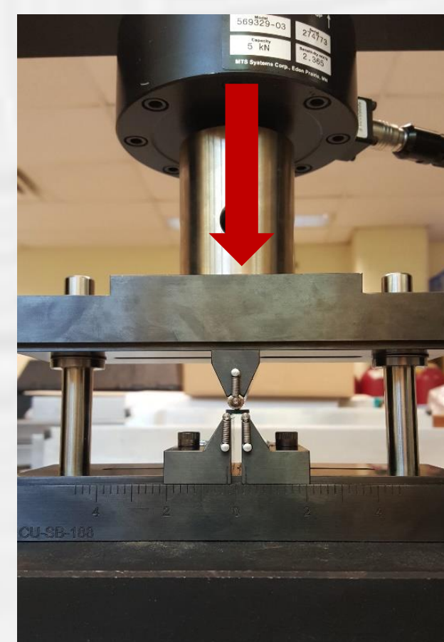
Three point bending fixture (ASTM D2344)
