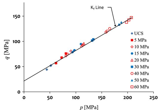
**Fig. 3** Results of triaxial tests conducted using the Obert–Hoek Cell—the axis of the test specimen is aligned normal to the nominal plane of the argillaceous partings (Selvadurai 2017)
