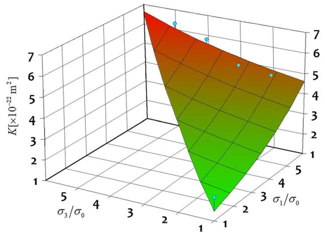
**Fig. 14** Estimates for the permeability evolution during stress release
