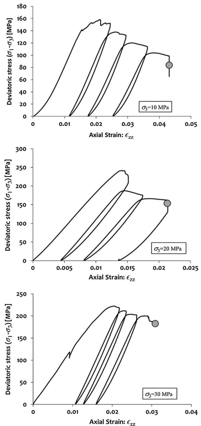
**Fig. 7** Typical results for the variation of deviatoric stress applied to the sample with axial strain (*filled circle* indicates the deviatoric stress level at which permeability tests are performed)
