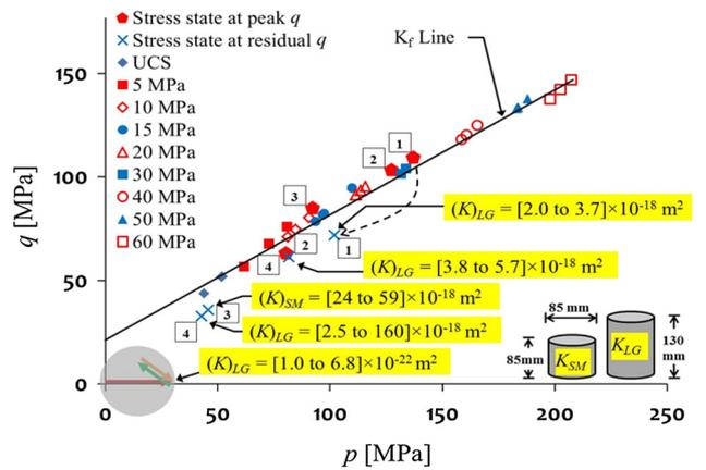
**Fig. 15** The post-failure permeability of the Cobourg Limestone
