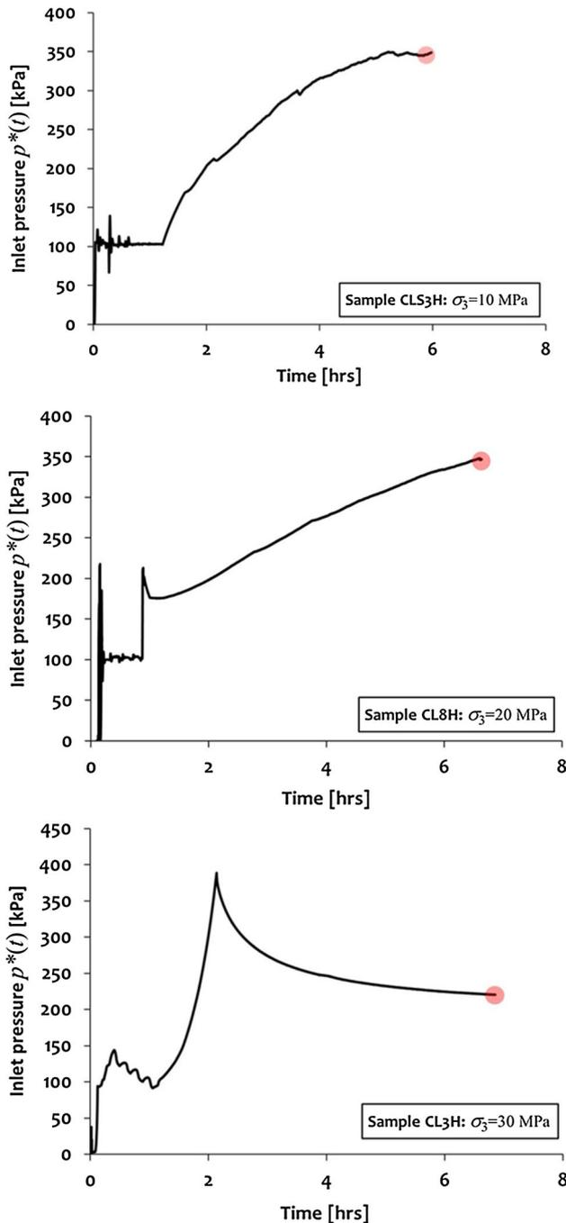
**Fig. 8** Time history of the entry point fluid pressure during steady-state permeability tests on failed samples (*filled red circle* indicates the inlet pressure at which steady-state permeability tests are performed) (colour figure online)
