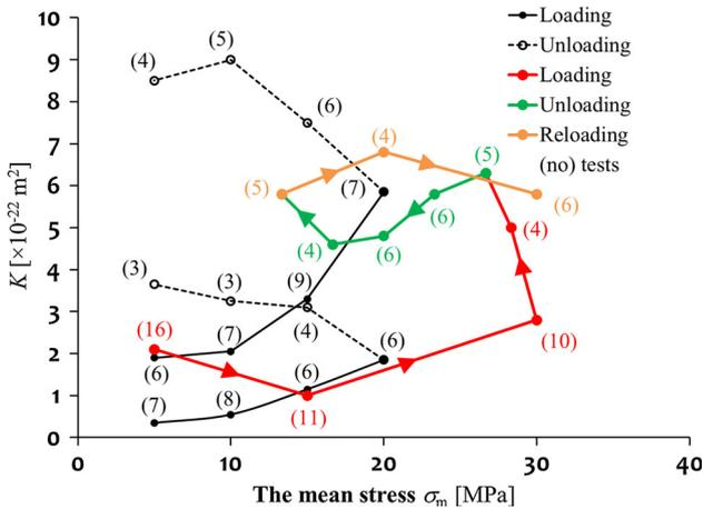
**Fig. 13** Permeability evolution of the Cobourg Limestone in pre-failure stress states as a function of the mean stress  $\sigma_m = (\sigma_1 + 2\sigma_3)/3$  (the solid and dotted black lines refer to the results obtained by Selvadurai et al. (2011))
