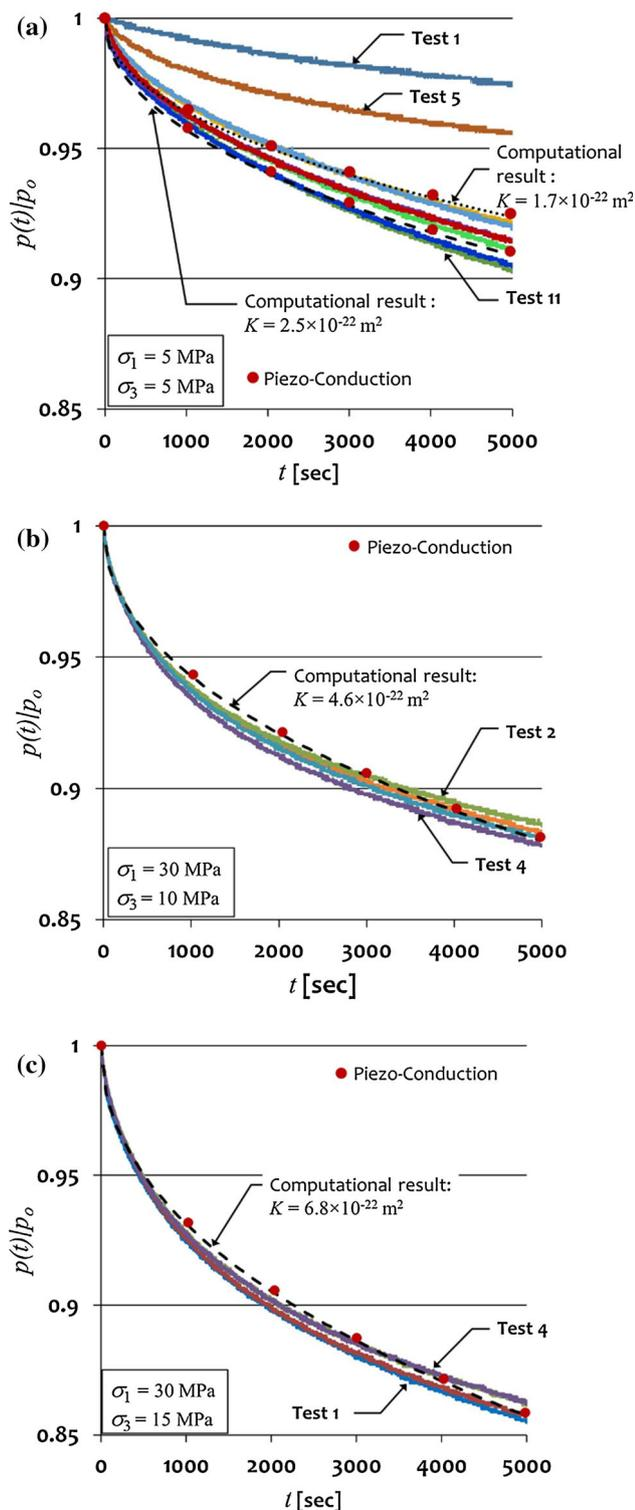
**Fig. 5** Typical cavity pressure decay patterns during hydraulic pulse testing of triaxially stressed Cobourg Limestone cylinders: **a** isotropic compression, **b** unloading with  $\sigma_1 = \text{constant}$  and **c** reloading with  $\sigma_1 = \text{constant}$
