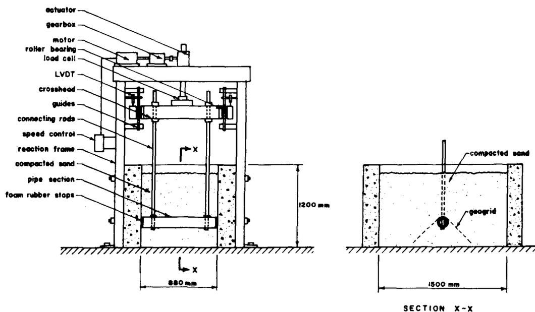
FIG. 2—A schematic view of the test facility.
