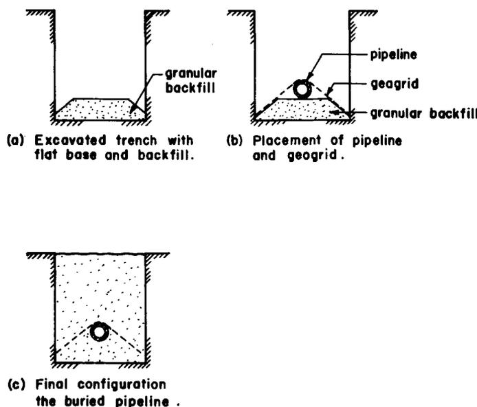
FIG. 5—A procedure for the installation of the geogrid.
