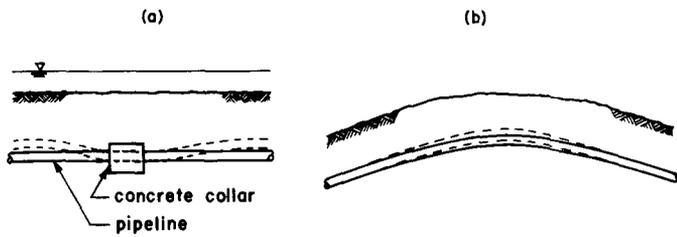
FIG. 1—Uplift action in buried pipelines: (a) effects of a floatation force and (b) overbend thrust caused by thermal or pressure effects.
