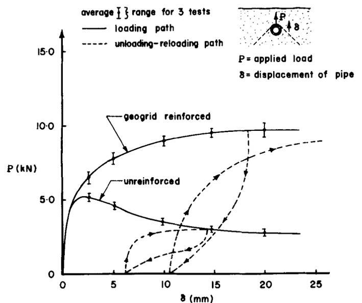
FIG. 4—Load-displacement behavior for the pipe section subjected to uplift loads. The influence of geogrid reinforcement.
