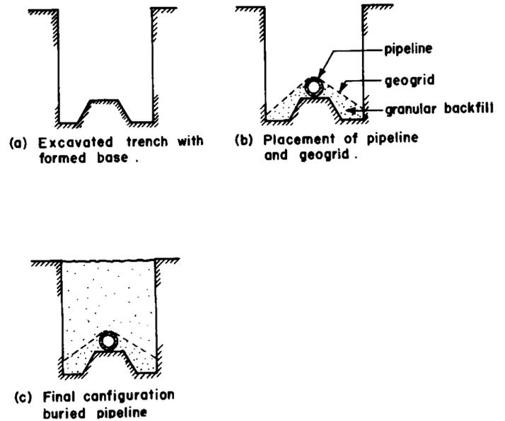
FIG. 6—A procedure for the installation of the geogrid.
