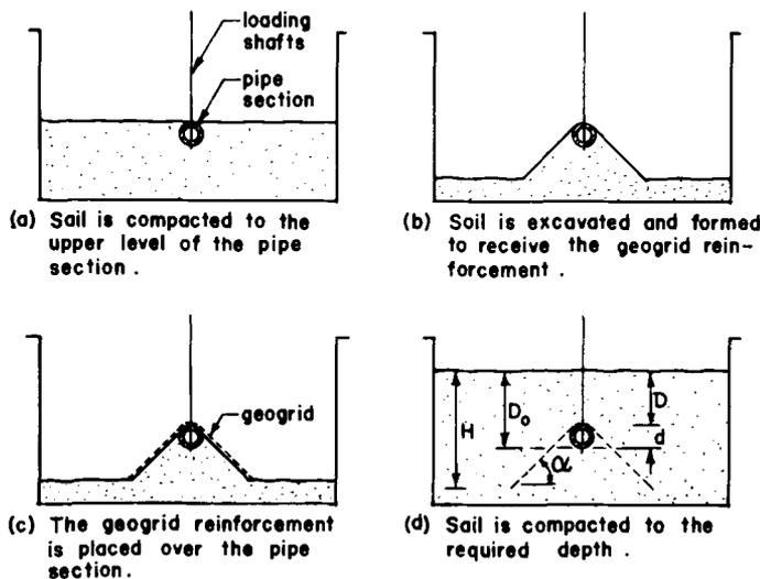
FIG. 3—Procedure for the installation of the pipeline and geogrid reinforcement.
