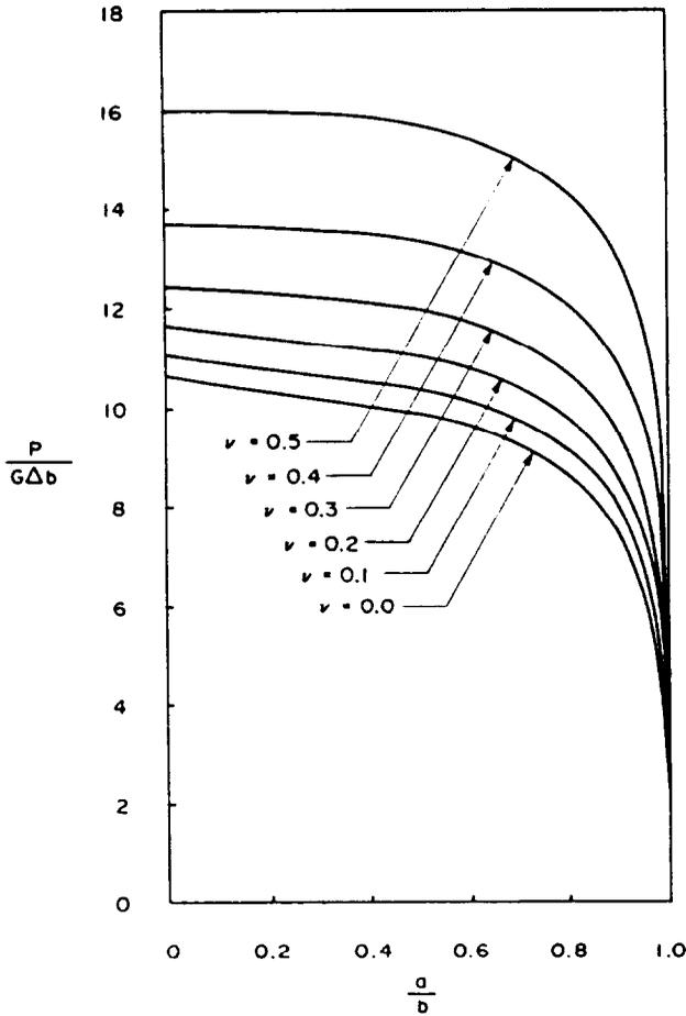
Fig. 2. The stiffness of debonded penny-shaped inclusion.
