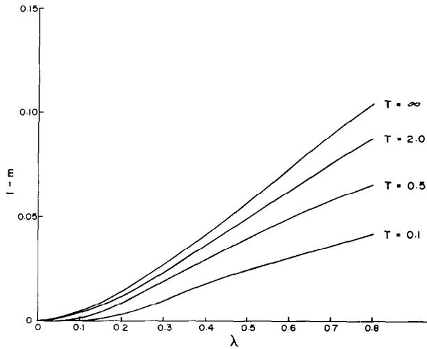
Fig. 2. Variation of length of plastic zone with  $\lambda$  for different values of  $T$  with  $\nu = \frac{1}{4}$ .
