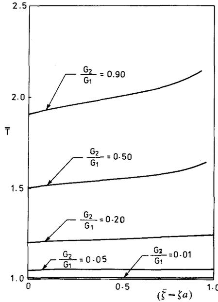
Fig. 2. Influence of the exponential non-homogeneity on the torsional stiffness of the rigid circular punch.
