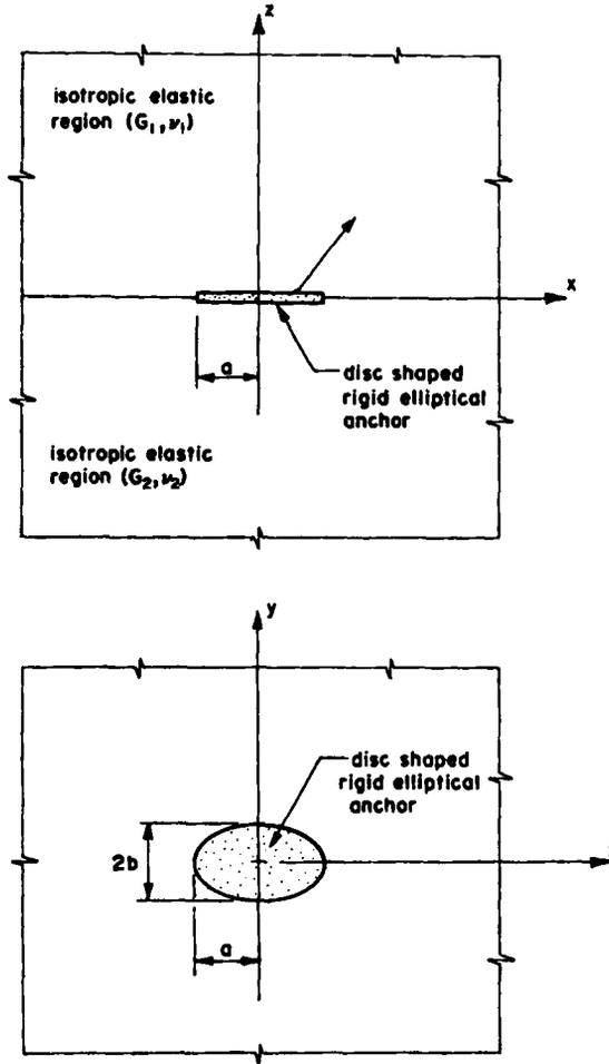
Figure 2. Rigid disc-shaped elliptical anchor region embedded at a bi-material elastic interface
