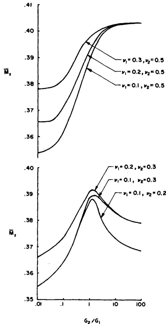
Figure 12. Torsional stiffness of a rigid elliptical anchor embedded at a bi-material geological interface
