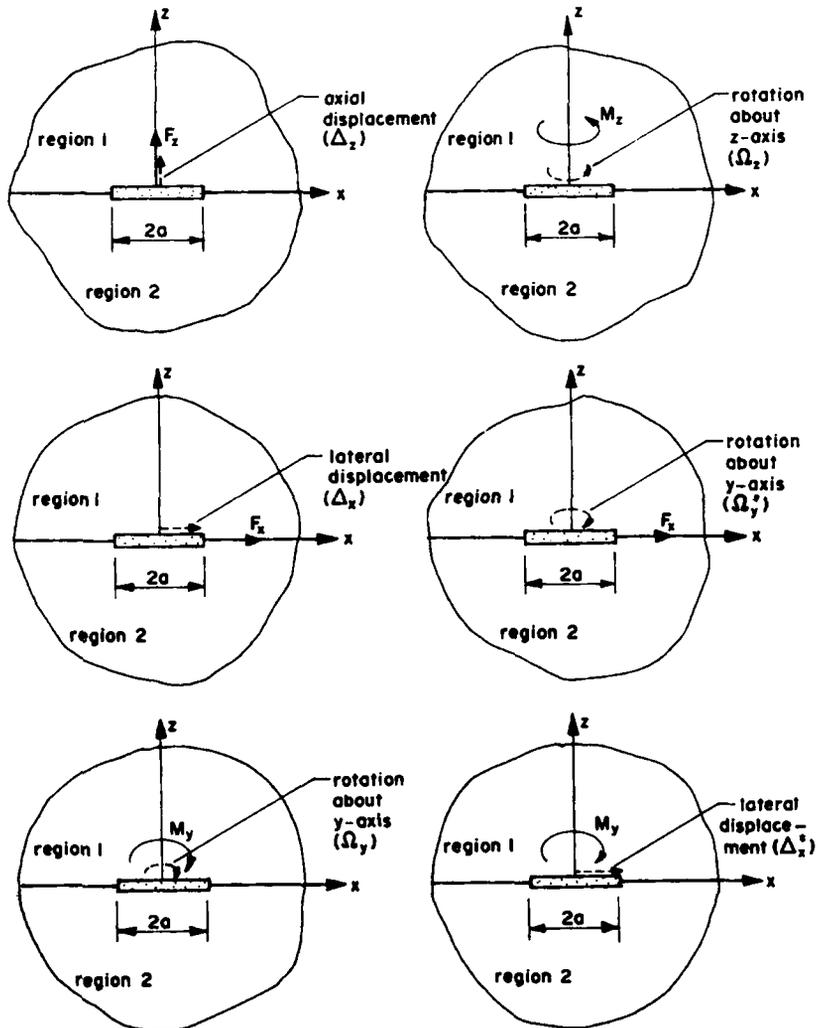
Figure 6. Generalized displacements of the elliptical anchor embedded at a bi-material geological interface
