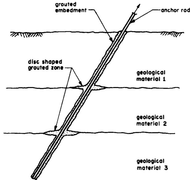
Figure 1. Disc-shaped anchor zones embedded at bi-material geological interfaces
