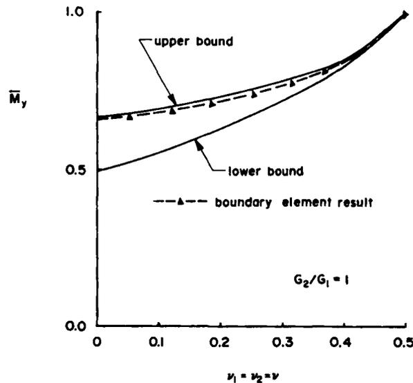
Figure 8. Rotational stiffness of a rigid elliptical anchor embedded in a homogeneous geological medium
