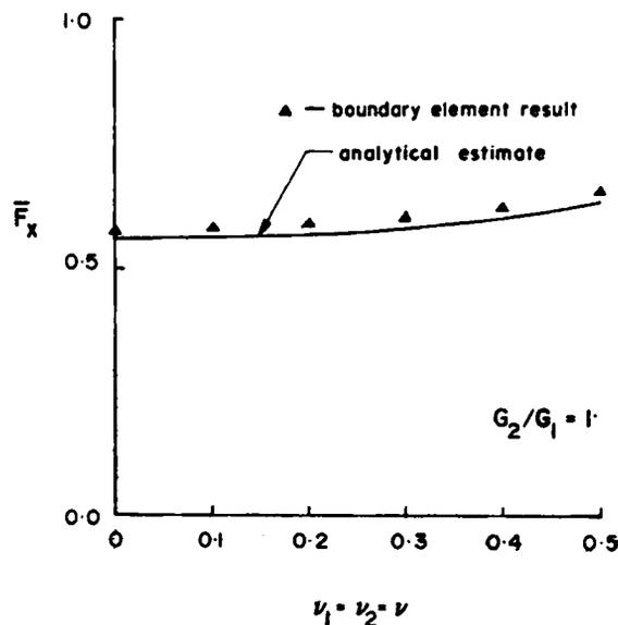
Figure 9. Lateral translational stiffness of a rigid elliptical anchor embedded in a homogeneous geological medium
