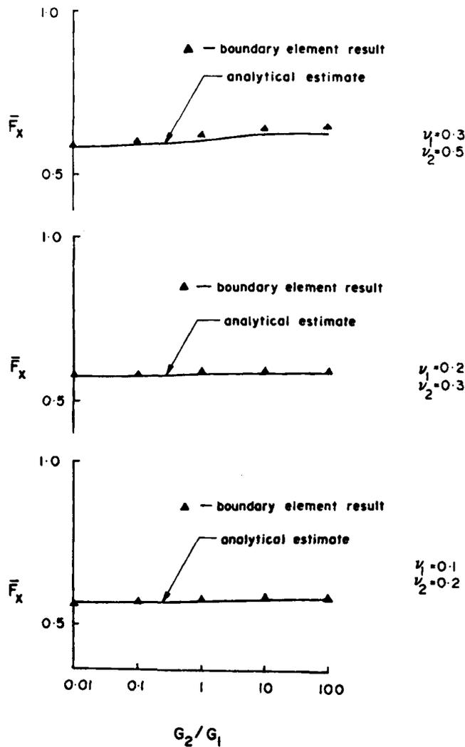
Figure 11. Translational stiffness of a rigid elliptical anchor embedded at a bi-material geological interface
