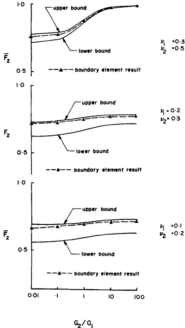
Figure 10. Axial stiffness of a rigid elliptical anchor embedded at a bi-material geological interface
