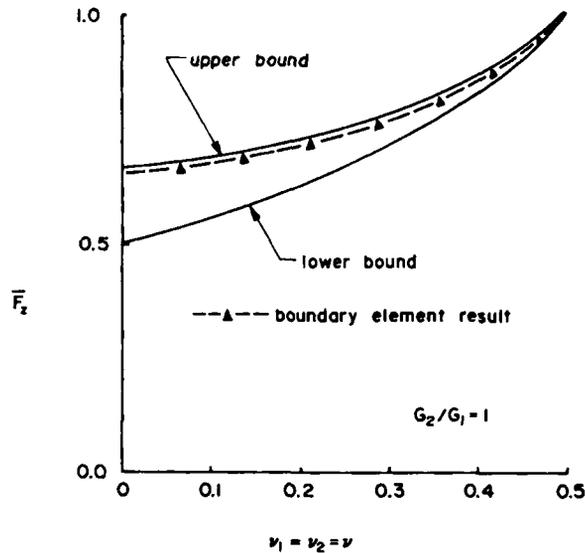
Figure 7. Axial stiffness of a rigid elliptical anchor embedded in a homogeneous geological medium
