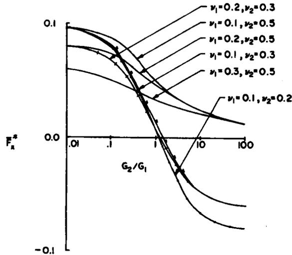
Figure 13. Coupling stiffness (rotation due to lateral force of a rigid elliptical anchor embedded at a bi-material geological interface)
