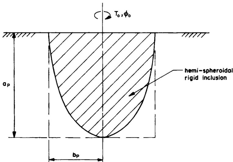
Figure 13. Geometry of hemi-spheroidal rigid inclusion
