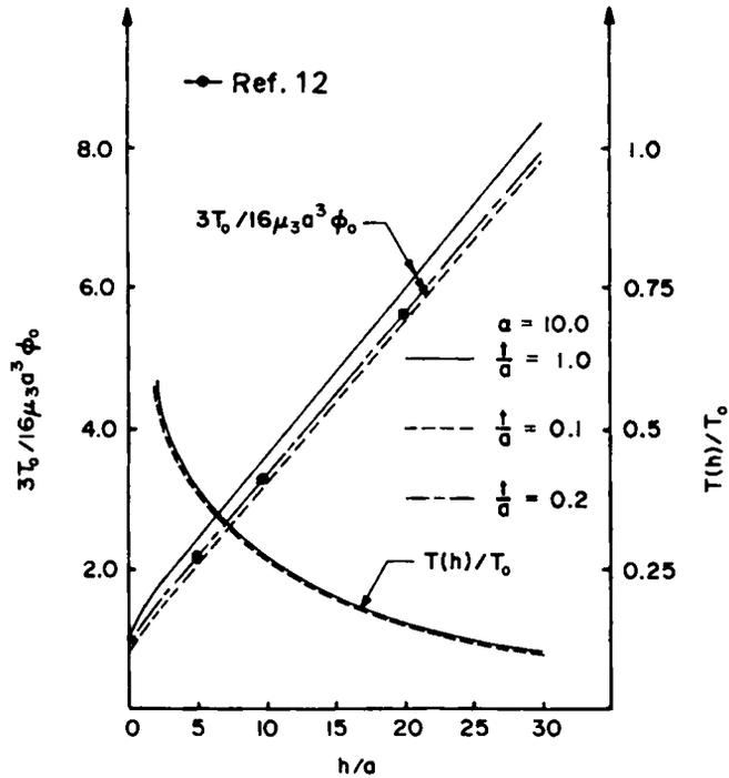
Figure 8. Variation of torsional stiffness and proportion of torque transfer at base for a hollow pier ( $\alpha = 10.0$ )
