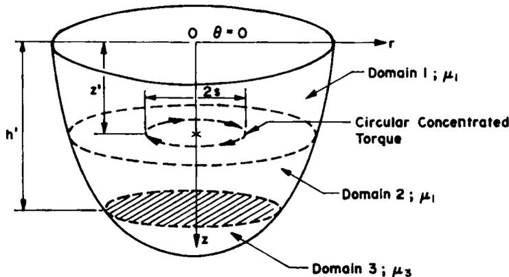
Figure 3. Circular concentrated torque in the interior of layered half space
