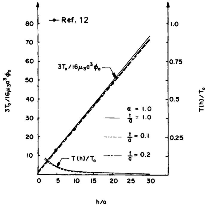
Figure 6. Variation of torsional stiffness and proportion of torque transfer at base for a hollow pier ( $\alpha = 1.0$ )
