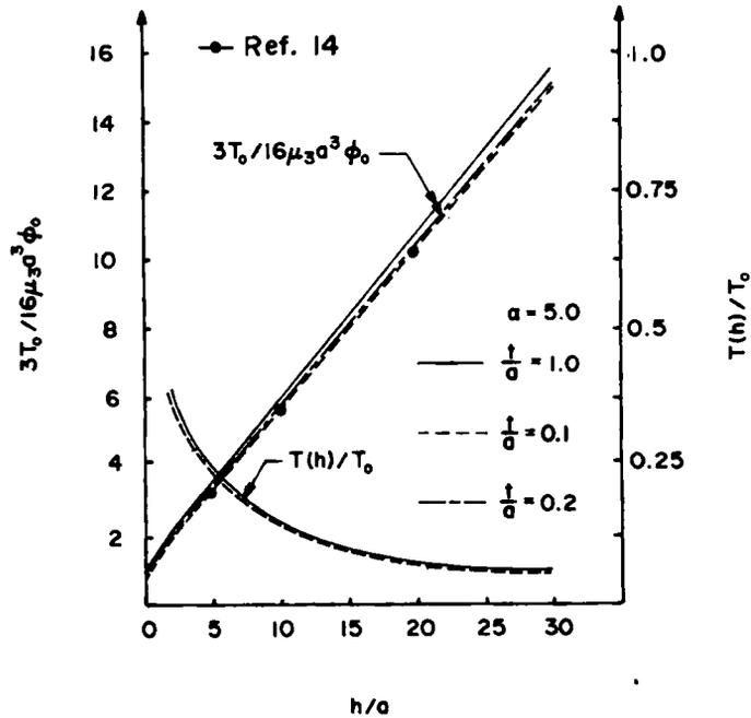
Figure 7. Variation of torsional stiffness and proportion of torque transfer at base for a hollow pier ( $\alpha = 5.0$ )
