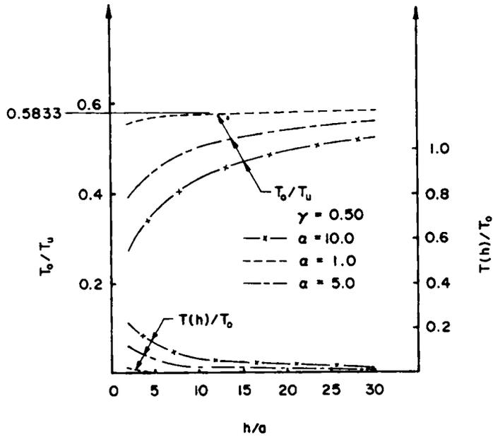
Figure 9. Variation of torsional stiffness and proportion of torque transfer at base for a tapered pier ( $\gamma = 0.50$ )
