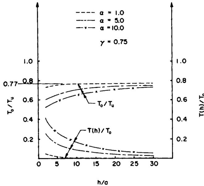
Figure 10. Variation of torsional stiffness and proportion of torque transfer at base for a tapered pier ( $\gamma = 0.75$ )
