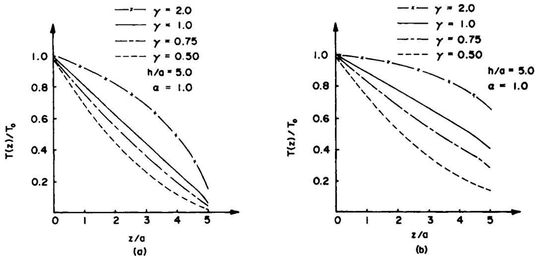
Figure 12. Torque transfer curves for a tapered rigid pier ( $h/a = 5.0$ )
