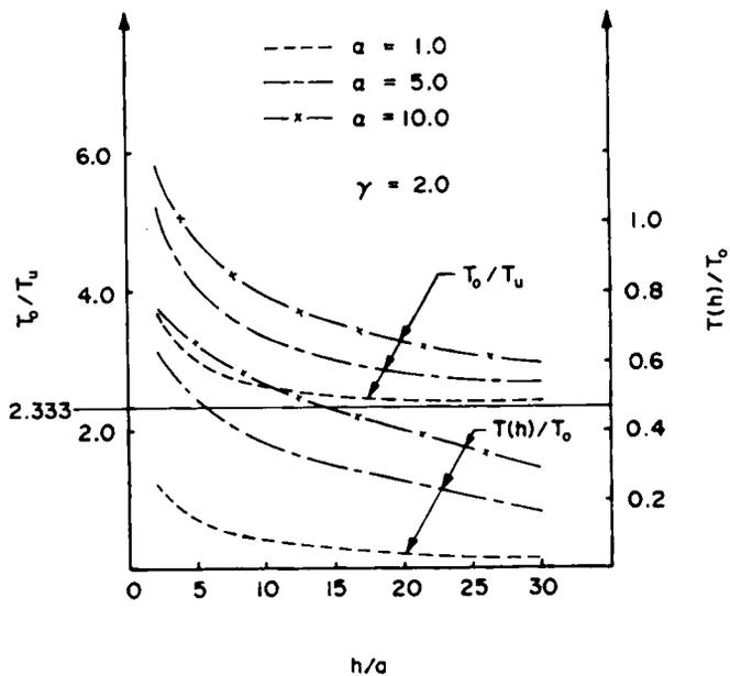
Figure 11. Variation of torsional stiffness and proportion of torque transfer at base for a tapered pier ( $\gamma = 2.0$ )
