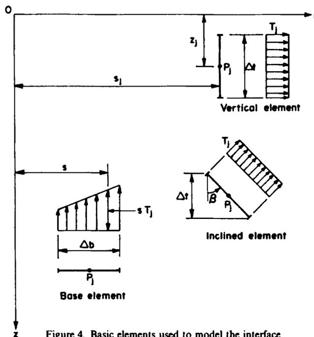
Figure 4. Basic elements used to model the interface
