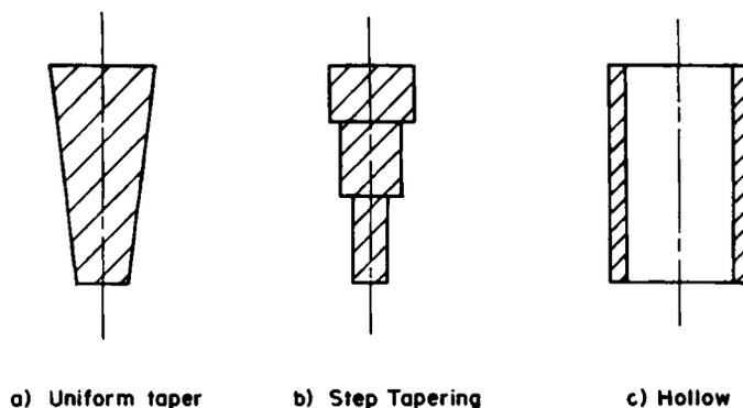
Figure 1. Rigid pier foundations
