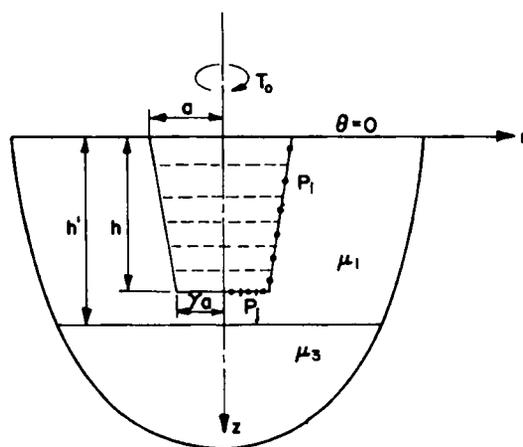
Figure 2. Discretization of a rigid pier
