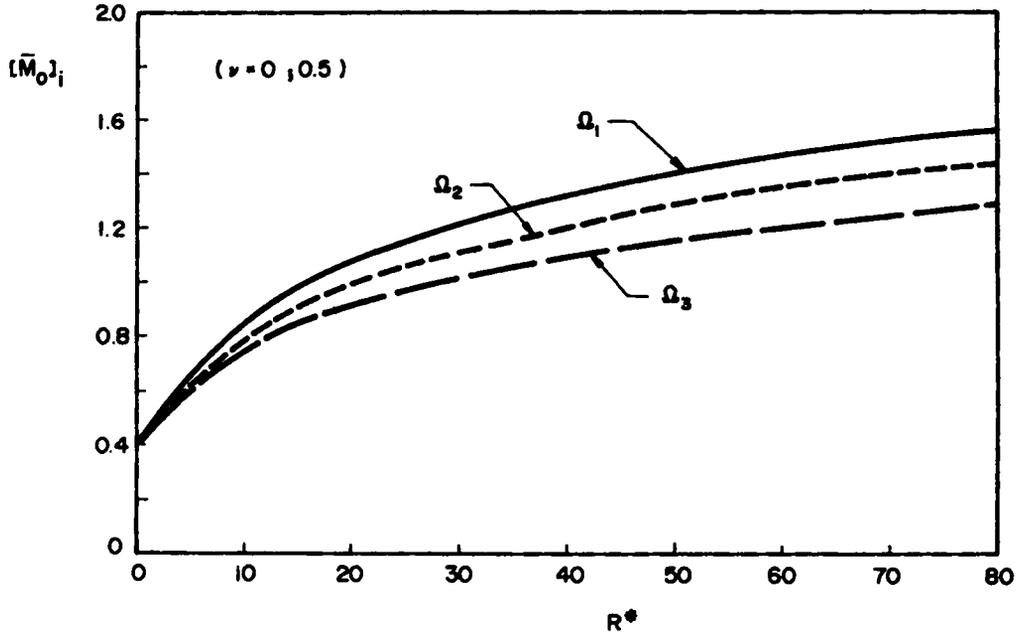
Figure 3. Variation in the maximum flexural moment in the embedded beam with the relative stiffness  $R^*$ :  $[\bar{M}_0]_i = [M(0)/P_0b/\pi]$ ;  $i = 1, 2, 3$
