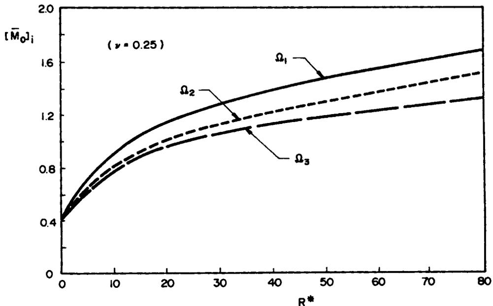
Figure 2. Variation in the maximum flexural moment in the embedded beam with the relative stiffness  $R^*$ :  $[\bar{M}_0]_i = [M(0)/P_0 b / \pi]_i$ ;  $i = 1, 2, 3$
