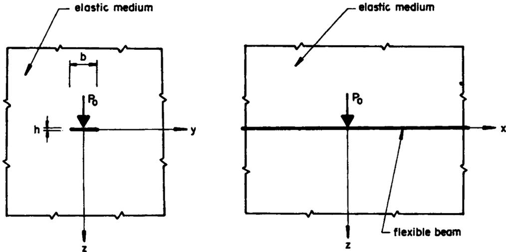
Figure 1. The geometry and loading of the embedded beam
