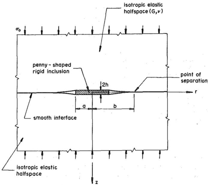
**FIG. 1.—Separation of Smooth Precompressed Interface by Smooth Rigid Disk Inclusion**
