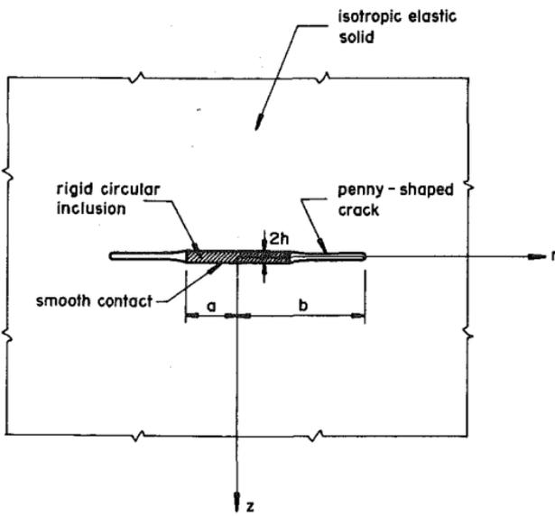
FIG. 2.—Indentation of Penny Shaped Crack by Smooth Rigid Disk Inclusion
