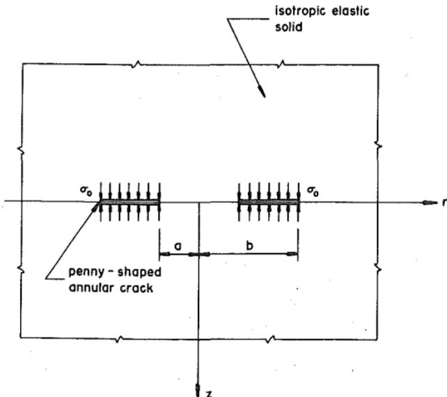
FIG. 3.—Geometry and Loading of Annular Crack
