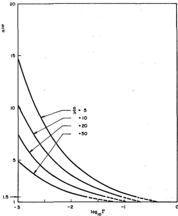
FIG. 4.—Influence of Precompression on Radius of Zone of Separation
