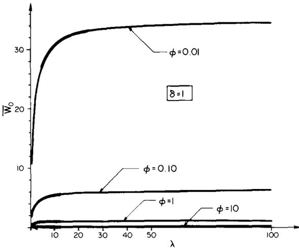
FIG. 2. Variation in the central deflection of the embedded beam.
