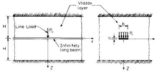
FIG. 1. Geometry of the infinitely long beam of finite width embedded in a Vlazov layer.
