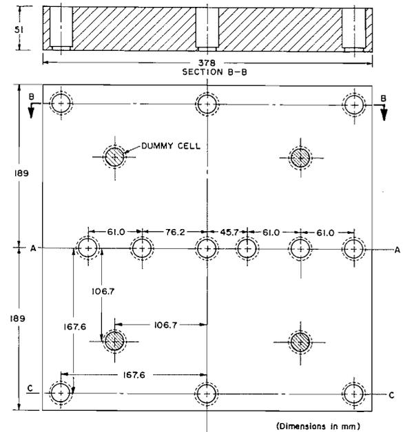
FIG. 5. The test plate and a configuration of contact stress transducers.
