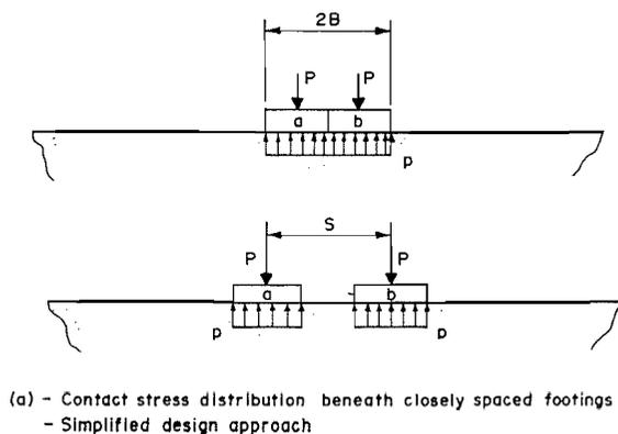
(a) - Contact stress distribution beneath closely spaced footings - Simplified design approach
