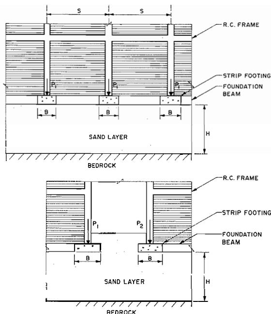
FIG. 1. Examples of mutual interference between strip foundations.
