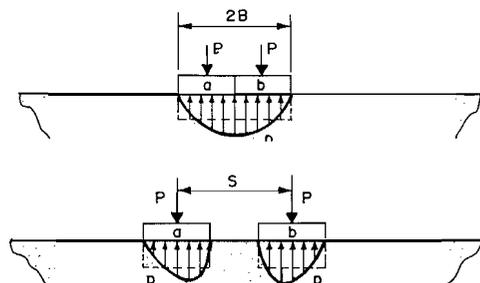
(b) - Contact stress distribution beneath closely spaced footings - Group effects
