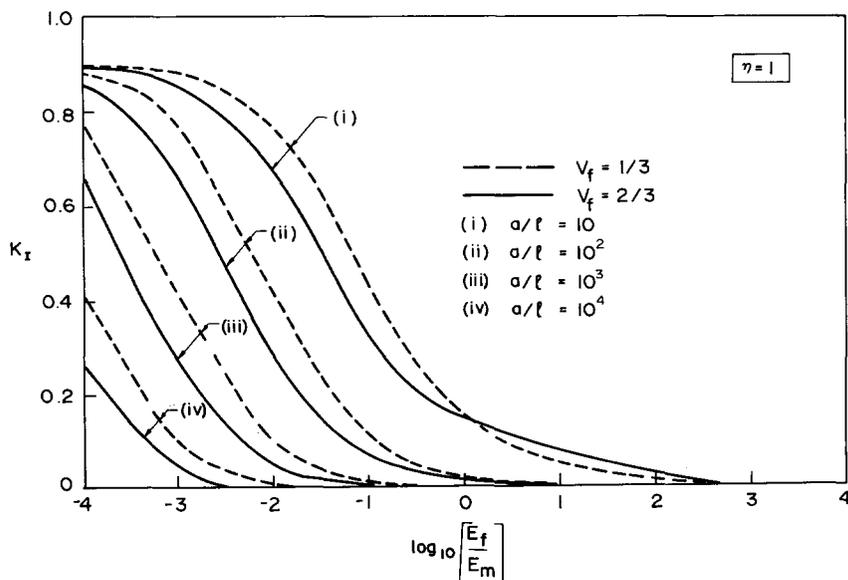
Figure 5. The normalized stress intensity factor  $\bar{K}_I$  for the bridged flaw.
