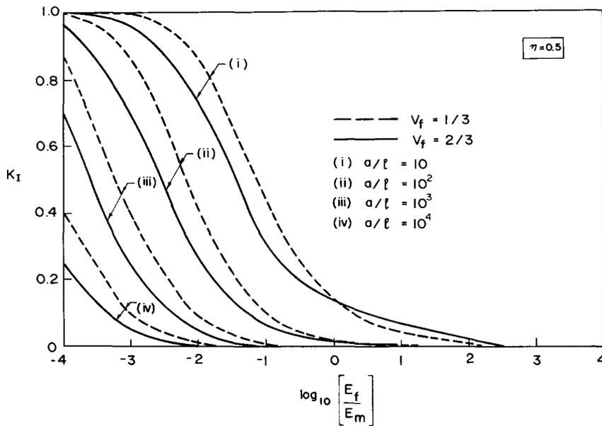
Figure 4. The normalized stress intensity factor  $\bar{K}_I$  for the bridged flaw.
