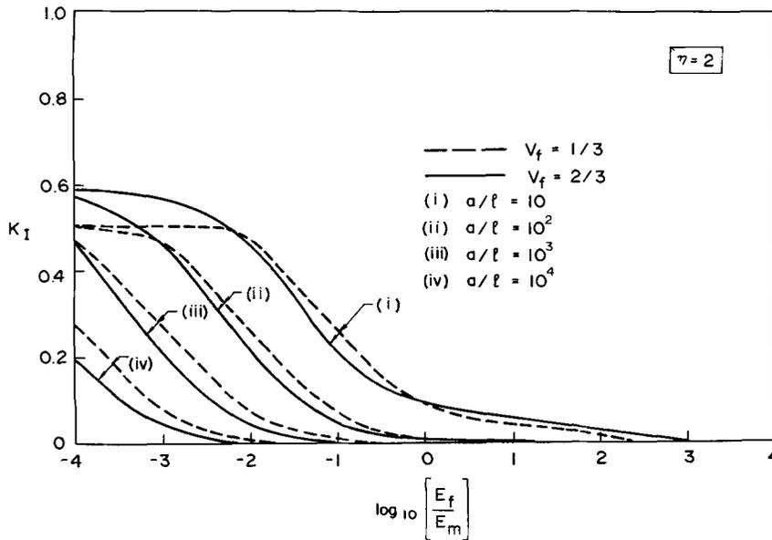
Figure 6. The normalized stress intensity factor  $\bar{K}_I$  for the bridged flaw.
