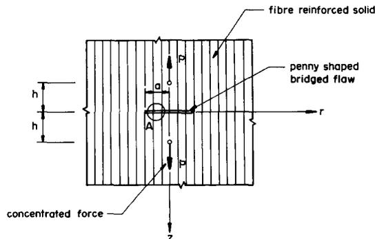
Figure 1. Geometry of the penny shaped flaw and the loading configuration.
