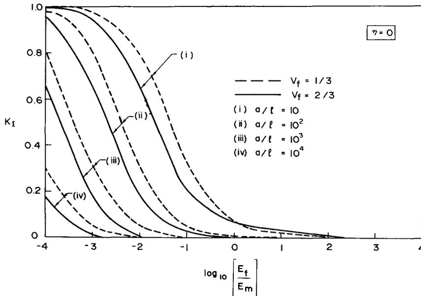
Figure 3. The normalized stress intensity factor  $\bar{K}_I$  for the bridged flaw.
