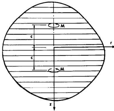
Fig. 2. Internal loading of the transversely isotropic infinite space.
