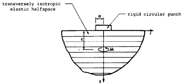
Fig. 1. The Reissner-Sagoci problem for an internally loaded halfspace.
