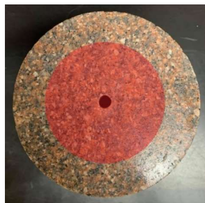
Figure 4. The sealed region (indicated in red) of the surface of the 150 mm diameter granite cylinder measuring with a cavity diameter of 10 mm.
