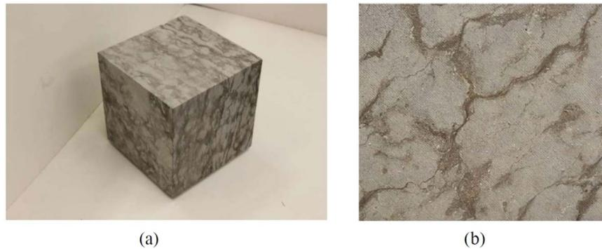
**Figure 1.** The fabric of the Cobourg limestone. (a) The lighter nodular features in a 300 mm cuboid (b) the darker argillaceous partings over a 100 mm × 120 mm area.
