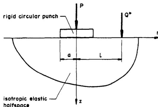
Fig. 1. Geometry of the rigid circular punch on an elastic halfspace and the external loading.
