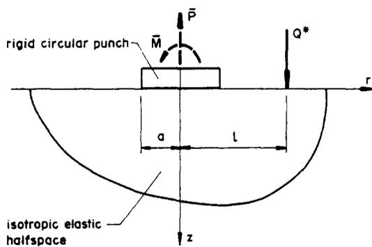
Fig. 2. Corrective force resultants
