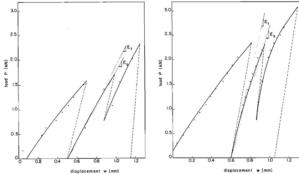
FIG. 5. Load-settlement curves for the screw plate test.
