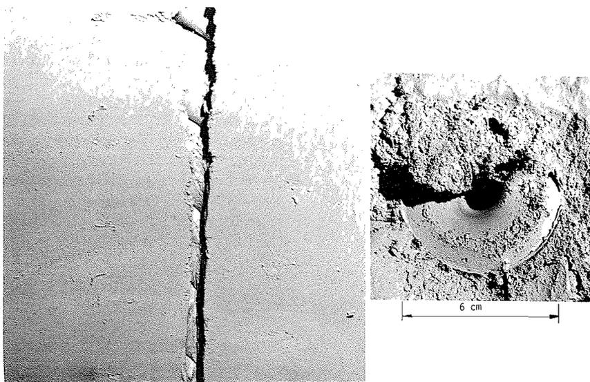
FIG. 2. Driven path of a model screw plate in compacted kaolin.
