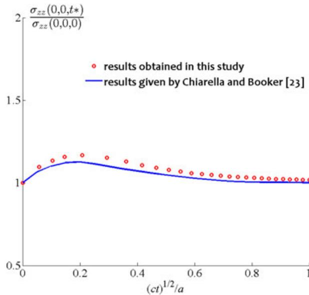
Figure 3. Comparison of the contact stress ratio at the centre of a rigid circular foundation with results given by Chiarella and Booker [23].
