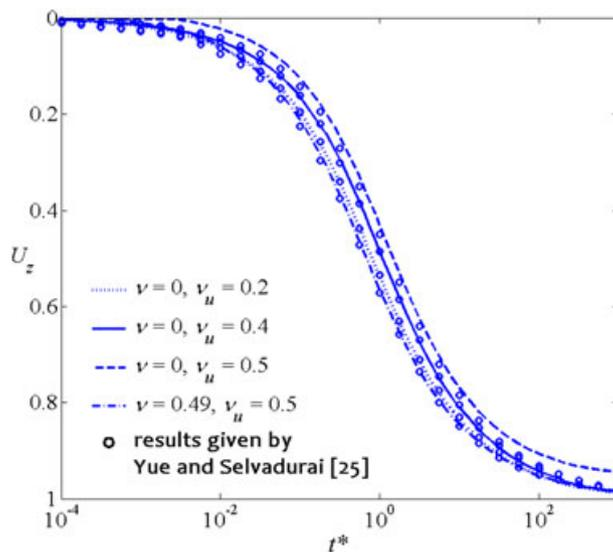
Figure 6. Consolidation rates for different Poisson’s ratios when *the surface is completely impervious*.
