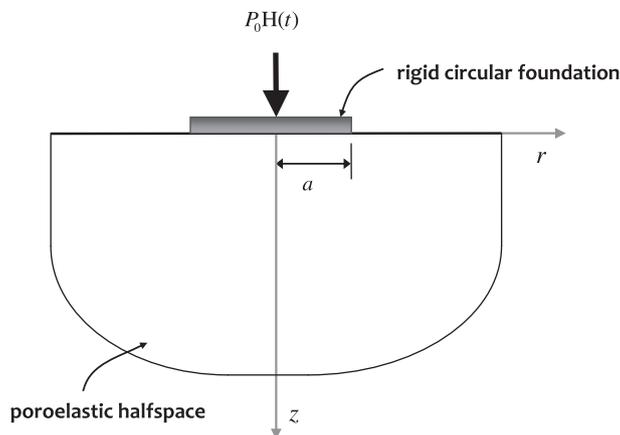
Figure 1. Indentation of a poroelastic halfspace.
