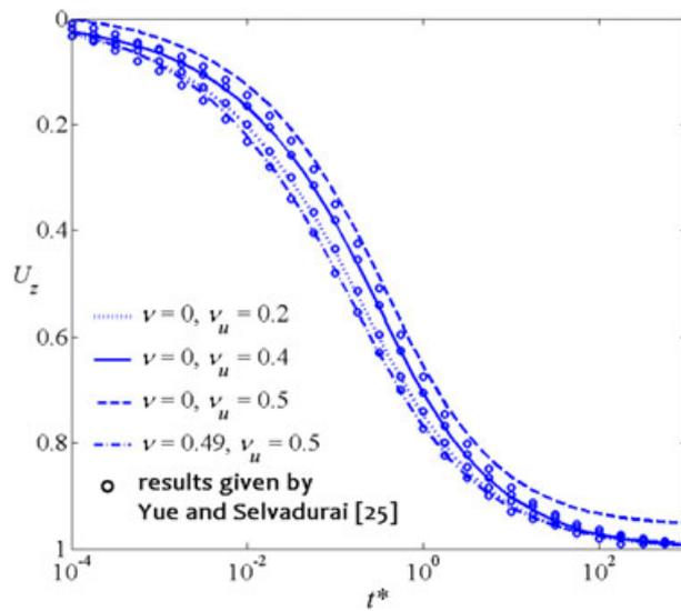
Figure 5. Consolidation rates for different Poisson’s ratios when *the surface is completely pervious*.
