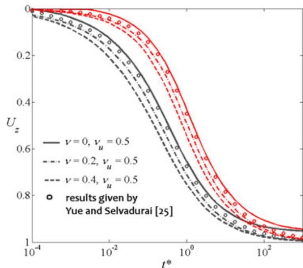
Figure 4. Effect of the drainage condition on the consolidation rate: black colour indicates the results obtained for Case I (*completely pervious boundary*); red colour shows the results obtained for Case II (*completely impervious boundary*).
