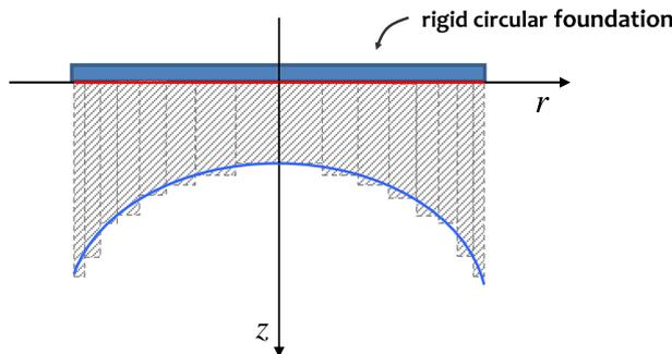
Figure 2. Discretization of contact loading by a rigid circular foundation.
