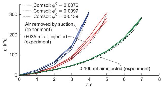
Fig. 13. Experimental results for the build-up of cavity pressure due to pumping water at the rate of  $Q = 2$  ml/min, for the three sets of hydraulic pulse tests performed on the Stanstead Granite sample
