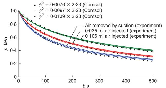
Fig. 14. Hydraulic pulse test results performed on the Stanstead Granite sample with three different air fractions
