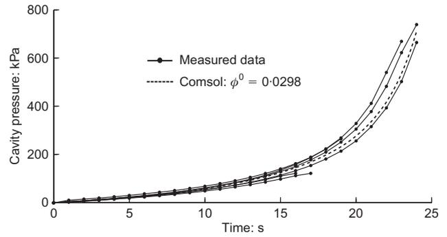
Fig. 11. Experimental results for the build-up of cavity pressure due to pumping water at the rate of  $Q = 2 \text{ ml/min}$ , for the Stanstead Granite sample
