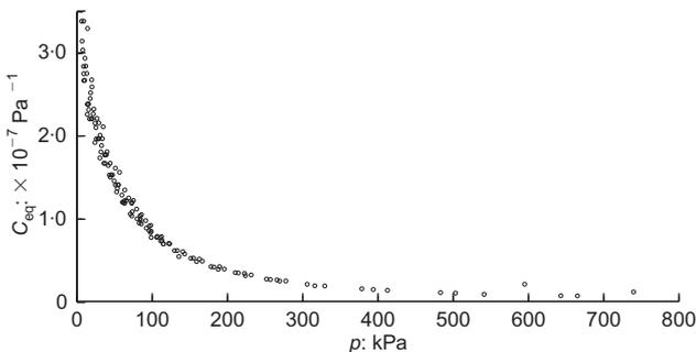
Fig. 10. Change of  $C_{eq}$  with cavity pressure increase in Stanstead Granite sample
