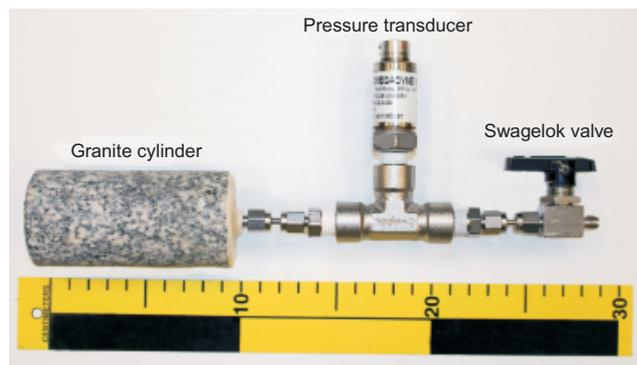
Fig. 5. The assembly of the Stanstead Granite sample
