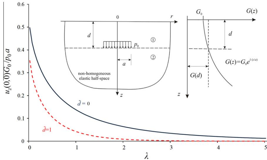
Fig. 4. Variation of the vertical displacement for different  $\lambda$ .
