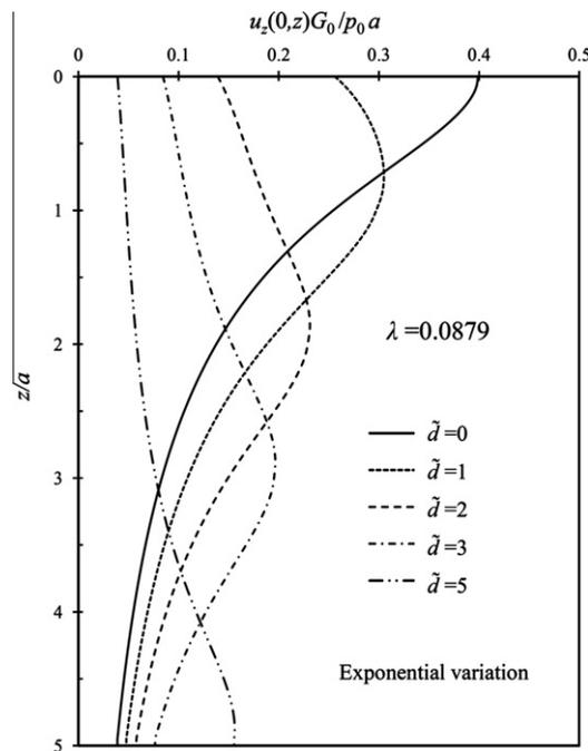
Fig. 10. Variations of vertical displacement along the z-axis for different depths of the loading for the fitted exponential variation of shear modulus to the data provided by Burland et al. (1977).
