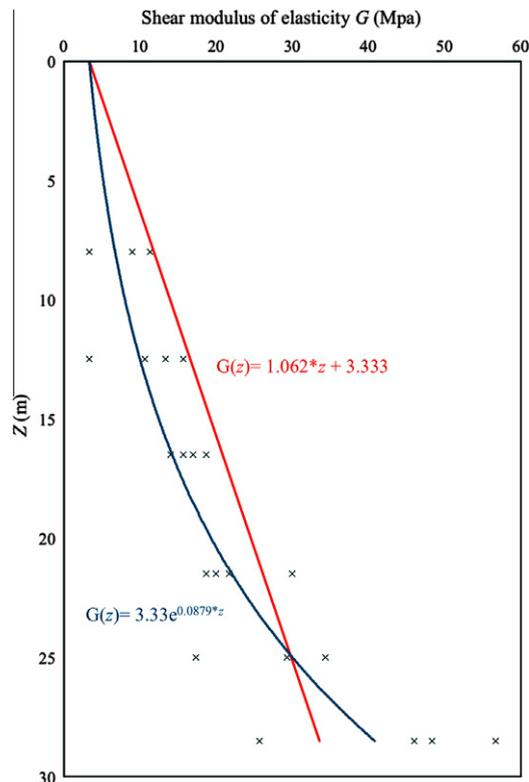
Fig. 2. Linear and exponential fit for the data provided by Burland et al. (1977).
