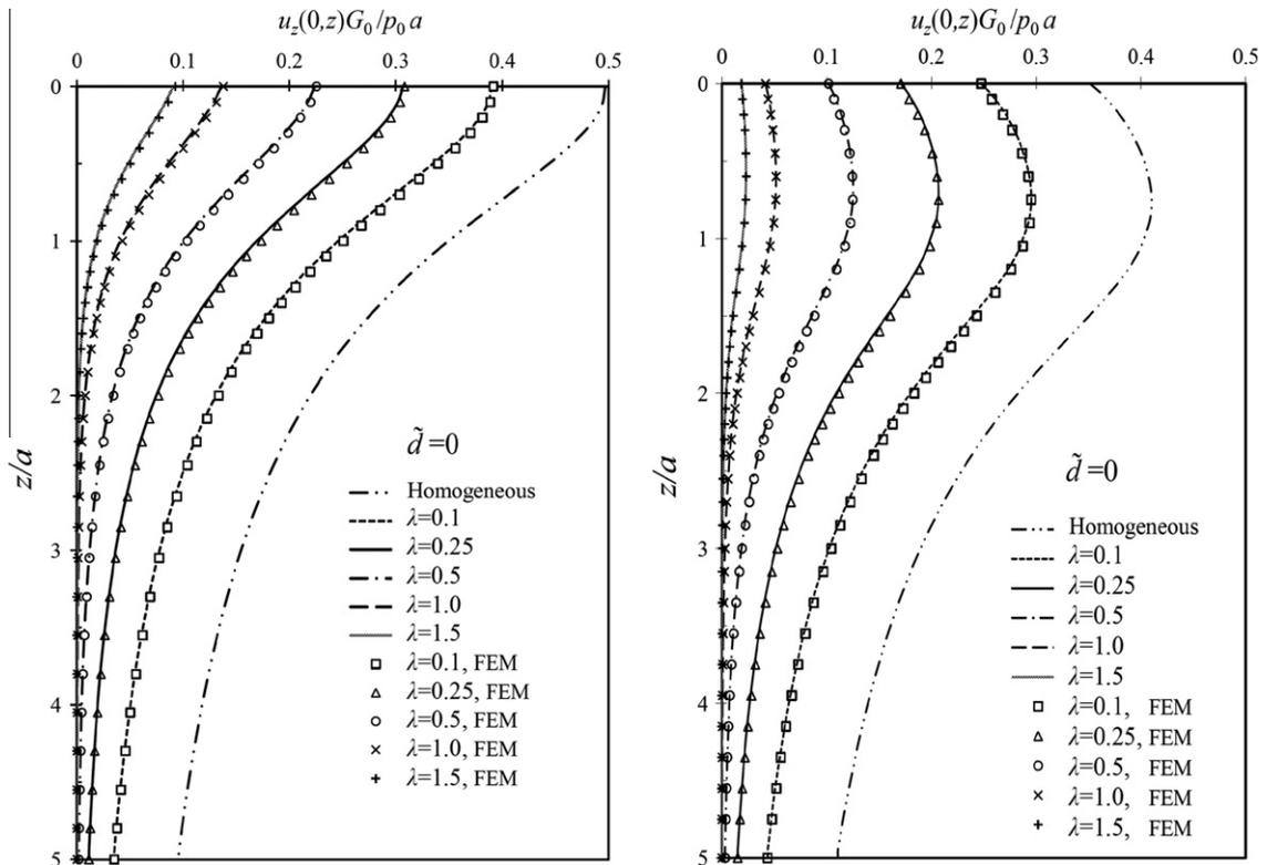
Fig. 7. Variation of the vertical displacement along the  $z$ -axis for different  $\lambda$  at depths  $\bar{d} = 0$  and  $\bar{d} = 1$ .
