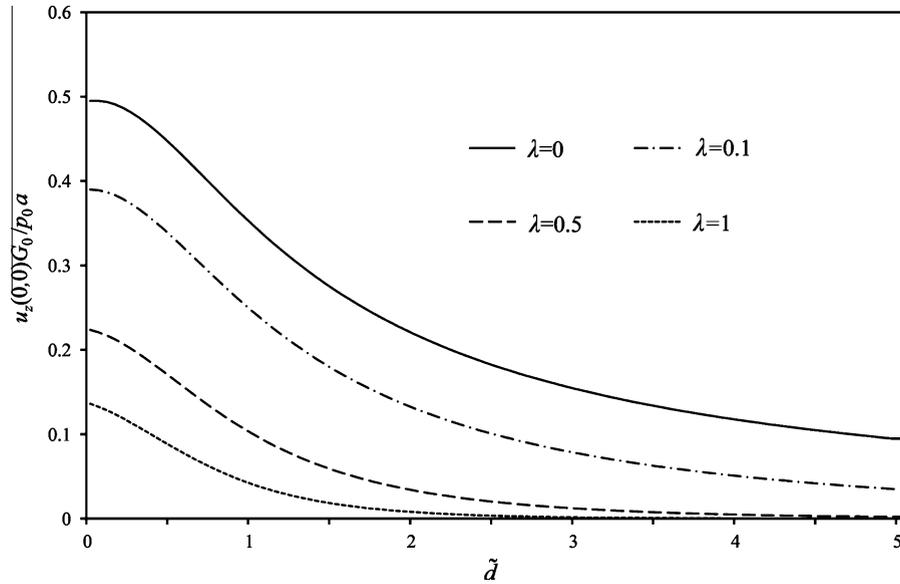
Fig. 5. Variation of the vertical displacement for different depth of loading ( $\tilde{d}$ ).
