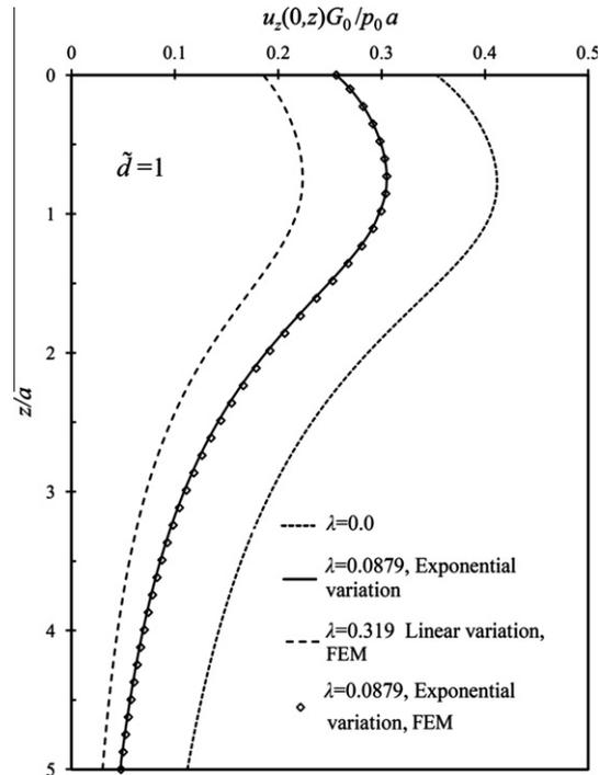
Fig. 9. Variations of vertical displacement along the  $z$ -axis for the fitted linear and exponential variation of shear modulus to the data provided by Burland et al. (1977).
