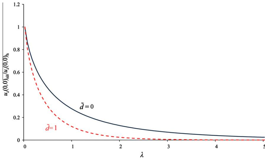
Fig. 6. Ratio of displacement in a non-homogeneous medium to a homogeneous medium for different  $\lambda$ .
