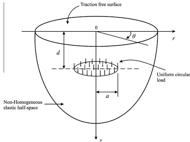
Fig. 1. Axisymmetric Mindlin loads acting at the interior of an incompressible non-homogeneous elastic half-space.
