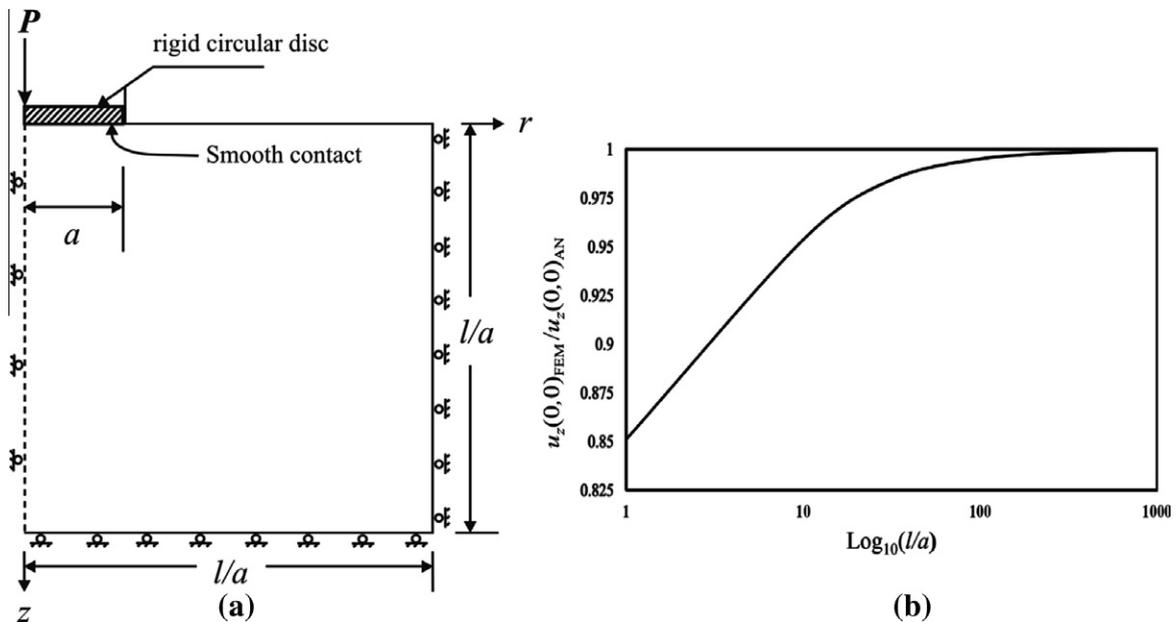
Fig. 3. (a) Finite element representation of the classic problem of the indentation of the surface of a rigid circular disc. (b) Vertical displacement for different  $l/a$ .
