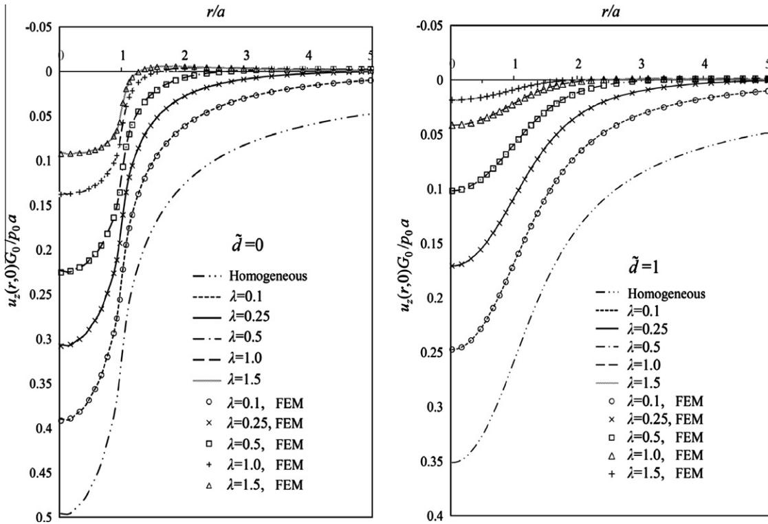
Fig. 8. Variation of the vertical displacement along the  $r$ -axis for different  $\lambda$  at depths  $\tilde{d} = 0$  and  $\tilde{d} = 1$ .
