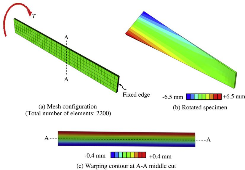
Fig. 5. Mesh configuration and deflection contours of SC-90° specimen due to  $T = 10.0 \text{ N.m}$ .
