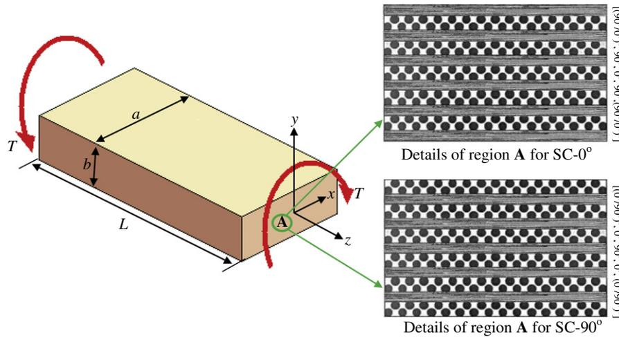
Fig. 1. Coordinate and dimensions of rectangular bar for Lekhnitskii model and details of strip lay-up at region A.
