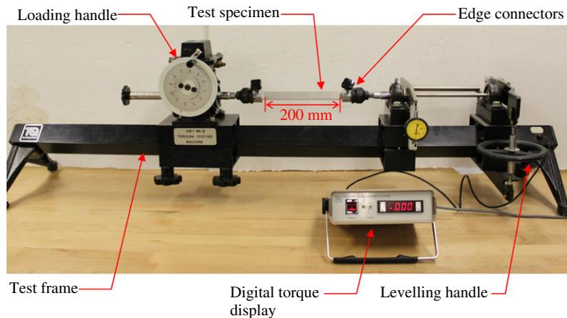
Fig. 3. Static torsion test setup.
