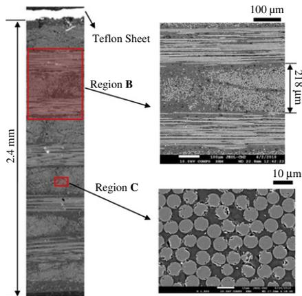
Fig. 2. Fibre arrangement as observed from a scanning electron microscope.
