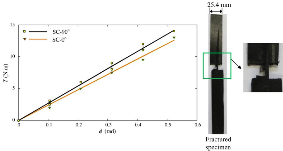
Fig. 4. Torque versus rotation curves and a typical fractured CFRP specimen.
