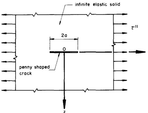
Fig. 1. The geometry of the penny-shaped crack
