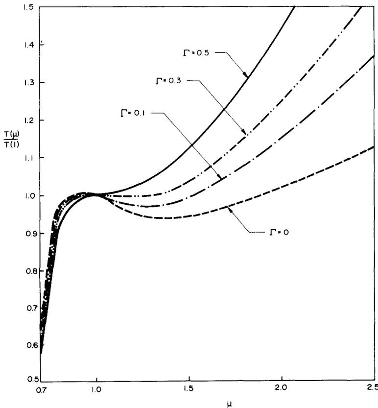
Fig. 2. The variation in the rupture stress of the penny-shaped crack with the initial finite deformation
