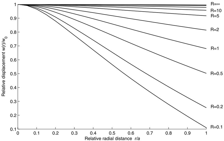
**Fig. 8** Relative plate displacements along  $0 \leq r \leq a$  for  $v_S = 0.3$  and  $P_M = P_0$  applied at  $c = a$
