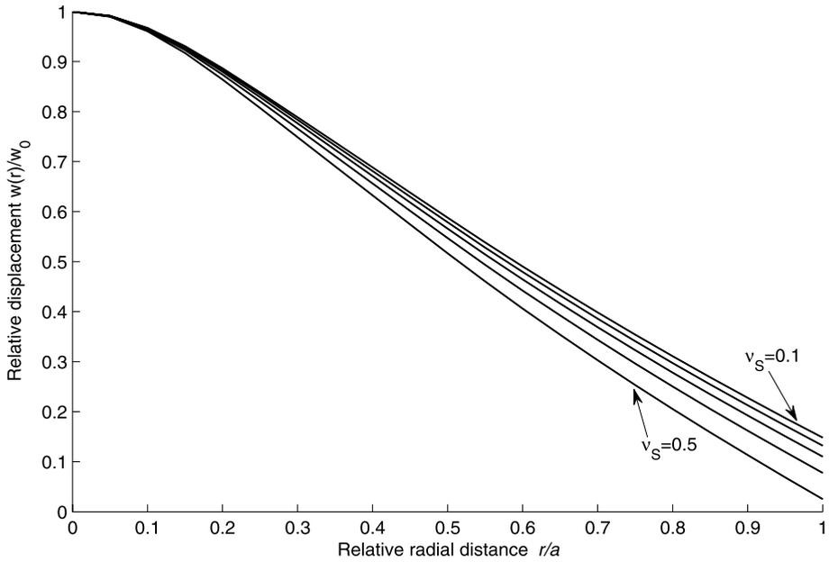
**Fig. 7** Relative plate displacements along  $0 \leq r \leq a$  for  $R = 0.1$  and  $P_M = P_0$  applied at  $c = a$
