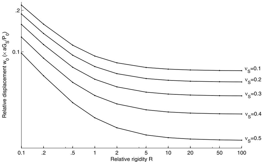
**Fig. 4** Displacements  $w_0$  of (16) for  $P_M$  applied at  $c = a$  and using  $m = 10$  terms in (5)
