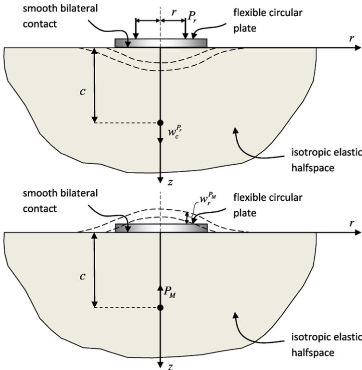
**Fig. 2** The reciprocal states: (a) displacement  $w_c^{P_r}$  at  $(r = 0, z = c)$  due to a ring force  $P_r$  on the plate at  $(r, z = 0)$ ; (b) displacement  $w_r^{P_M}$  at  $(r, z = 0)$  due to a point force  $P_M$  at  $(r = 0, z = c)$
