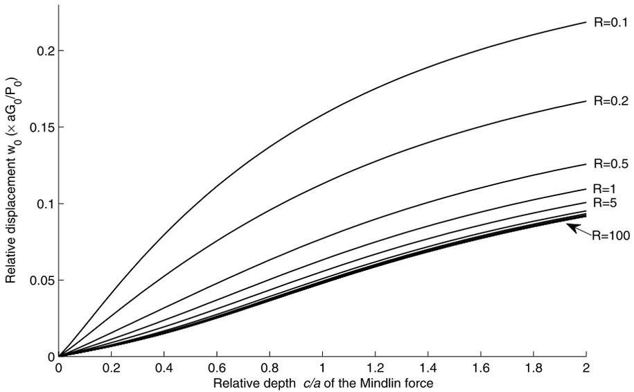
**Fig. 5** Displacements  $w_0$  of (16) for  $\nu_S = 0.3$  and using  $m = 10$  terms in (5)
