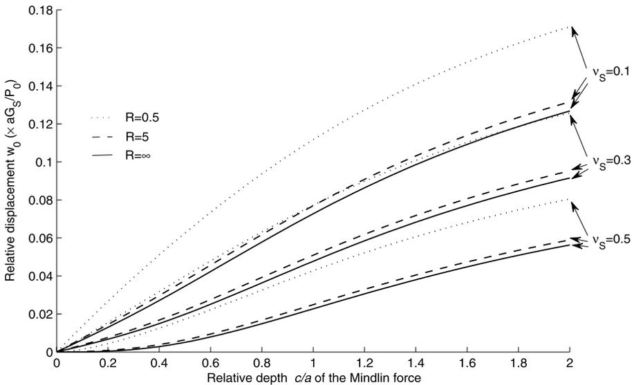
**Fig. 6** Displacements  $w_0$  of (16) for  $m = 10$  terms in (5) (dot, dash and solid line representations for the relative rigidity values  $R = [0.5, 5, \infty]$ )
