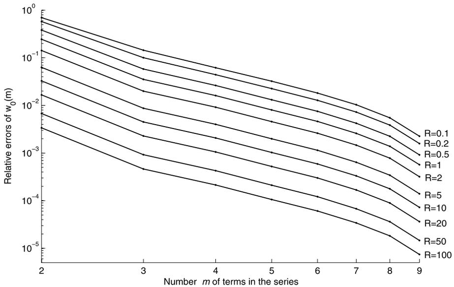
**Fig. 3** Relative errors of  $w_0$ , for  $m = 2, \dots, 9$  terms in (5), as referred to  $m = 10$  terms. The Mindlin force  $P_M$  is applied at the depth  $c = a$  and the Poisson's ratio is  $\nu_S = 0.3$
