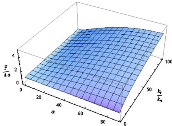
Figure 5. Influence of the orientation of the stratified porous medium and the hydraulic conductivity mismatch on the intake shape factor.
