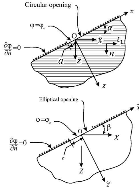
Figure 2. Transformation of the hydraulically transversely isotropic porous medium to a pseudo-isotropic medium.
