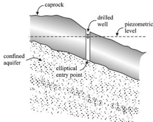
Figure 3. Borehole entry point that intersects an inclined interface.
