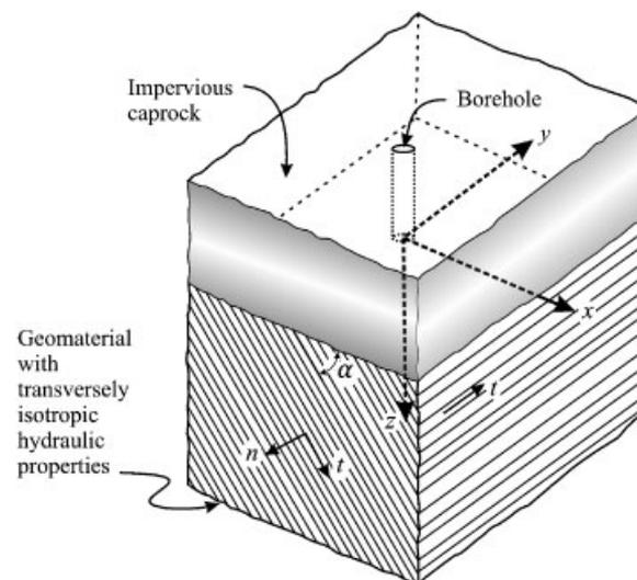
Figure 1. Borehole entry point at an interface with inclined stratification of the permeable medium.
