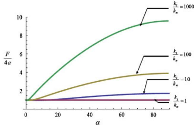
Figure 4. Influence of the orientation of the stratified porous medium on the intake shape factor.
