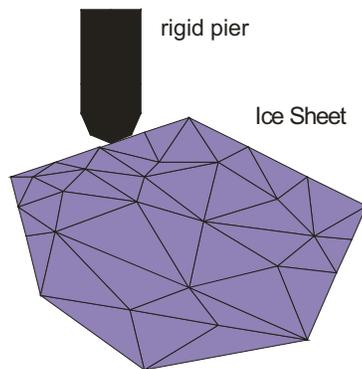
Figure 6: The finite element discretization used in the modelling of the intact ice sheet
