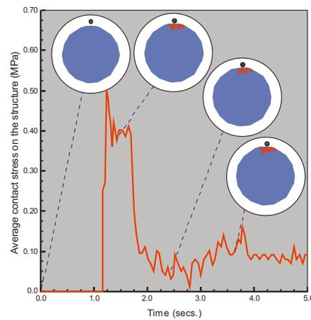
Figure 5: Time-dependent evolution of interactive contact stresses between the impacting ice-sheet and the stationary rigid pier - oblique impact.
