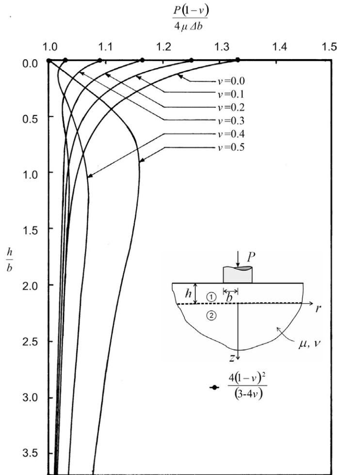
Fig. 2. Load–displacements response for a rigid indenter on an elastic halfspace containing an inextensible membrane.
