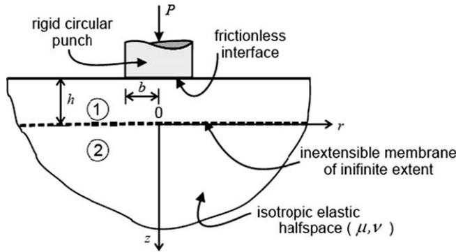
Fig. 1. The axisymmetric indentation of an elastic halfspace containing an inextensible circular membrane.
