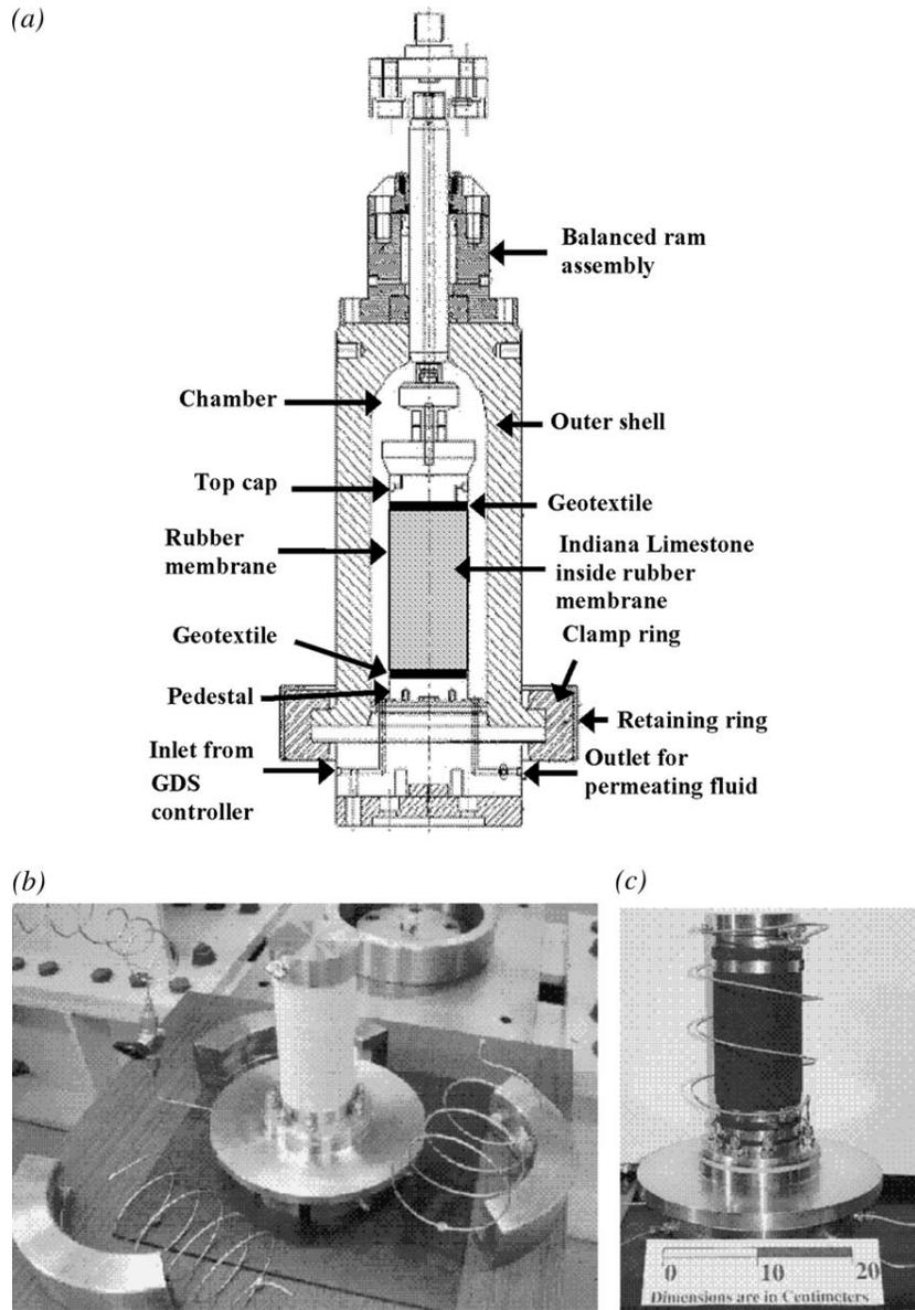
**Figure 1. Cross section of the high-pressure triaxial cell and assembly views of the sample setup.**
