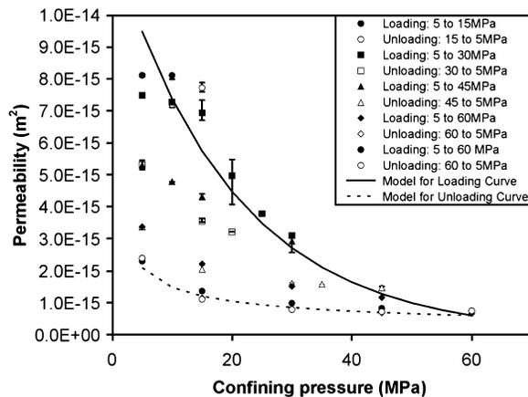
**Figure 5. Variation of permeability with isotropic stress history: Monotonic loading and unloading to the reference confining stress state (test C).**
