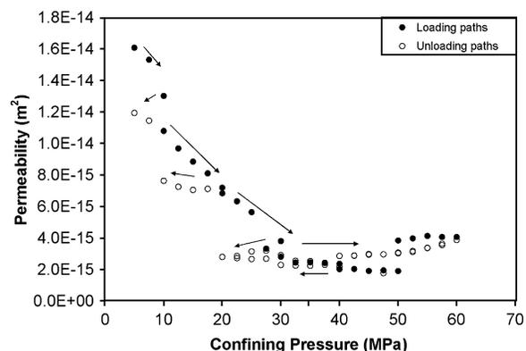
**Figure 3. Variation of permeability with isotropic stress history: Loading-partial unloading-reloading (test A).**
