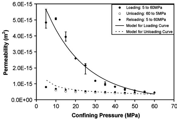
**Figure 4. Variation of permeability with isotropic stress history: Monotonic peak loading followed by complete unloading and reloading (test B).**
